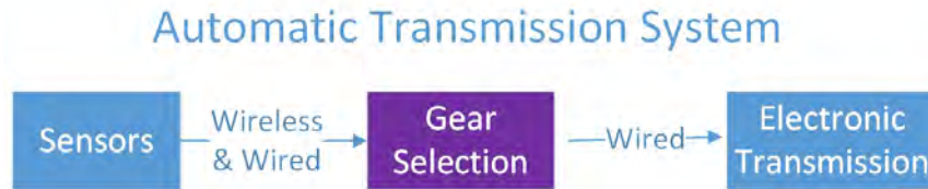
Figure 2.3: ATS consisting of a gear selection module, sensors and an ETS. The design of the GSS module and the communication to the ETS are the objectives of this report.
