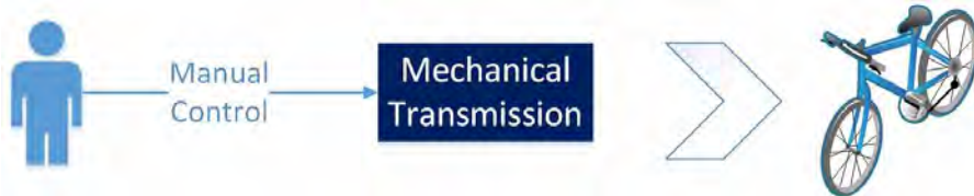
Figure 2.1: Overview of how traditional MTS and how it is operated by the user. Control levers are based on cable tension.
