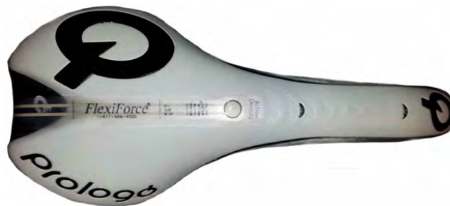
Figure 4: FlexiForce pressure sensor mounted on bicycle saddle using clear tape. Ideal location of the pressure sensitivity part of the sensor depends on the saddle type and rider. An area where relatively high pressure is applied on the saddle while sitting should be chosen.
