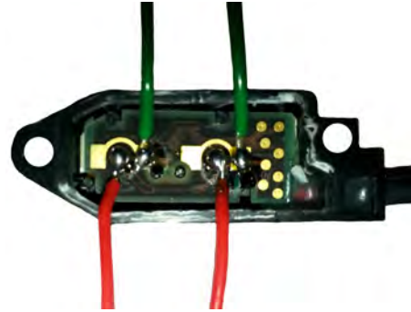
Figure 5.4: Disassembled button switch (SW-R671). Voltage across green and red contacts is +3.3V. Green wires were connected to common ground on DAQ device.
