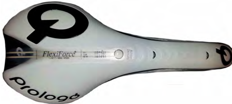
Figure 4.11: FlexiForce force sensor mounted on bicycle saddle using clear tape. The sensor presence is not noticeable while seated on the saddle. Here the pressure sensitive part of the sensor is located at the center of the saddle.
