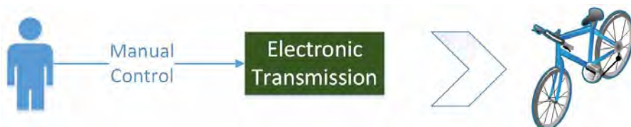
Figure 2.2: ETS is operated by the user in the same manner as traditional transmission. Control levers are based on electronic switches.
