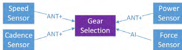
Figure 2.4: The GSS reads speed sensor, cadence sensor, power sensor and force sensor and uses the data to determine the optimal gear for the given situation and takes actions based on the multi-sensor data. In this context, processing of the multi-sensor data is defined data fusion.
