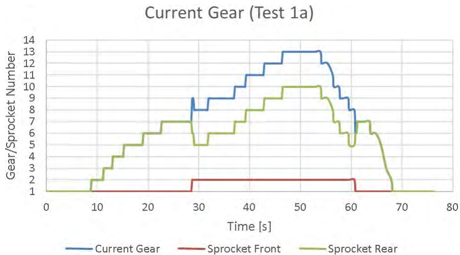
Figure 11.6: Graph showing G_C and corresponding combinations of S_F and S_R . Shifting between 7th and 8th gear requires 1 shift on the front derailleur and two shifts on the rear derailleur. This causes the system to temporarily go in a sprocket combination equivalent to 9th gear in the shifting sequence. This appears as a spike on the graph at t \approx 30s . The same occurs when shifting from 8th down to 7th gear, then the system is temporarily into a sprocket combination equivalent to 6th gear in the shifting sequence. This appears as a negative spike on the graph at t \approx 60s where G_C drops to 6 before reaching 7.
