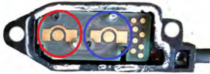
Figure 5.3: Disassembled button switch (SW-R671) (Sarti, 2013). Each colored ring shows the contacts for each button switch.
