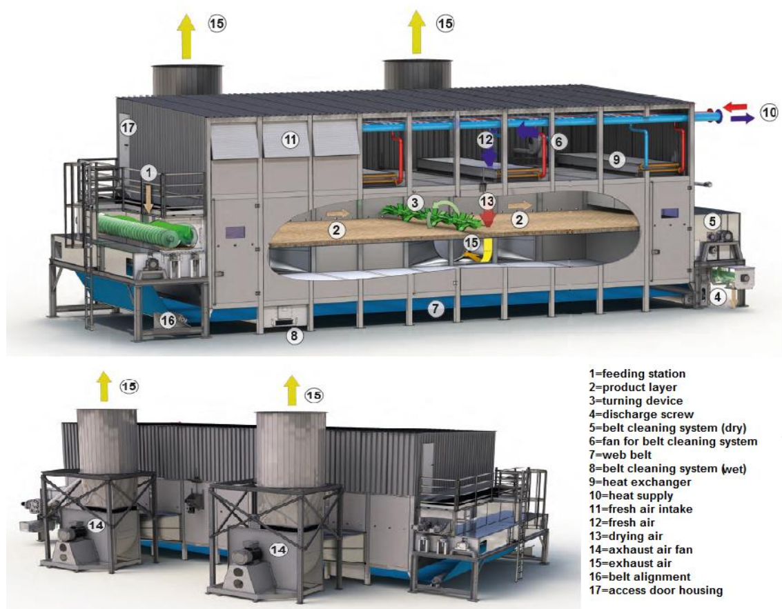
Figure 3-5 Belt dryer configuration for RDF drying[7]
