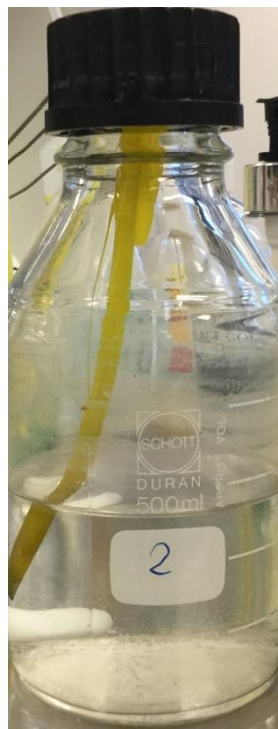
Figure 25 Formation of elemental sulphur in bottom reactor without biomass at T = 25\text{ }^{\circ}\text{C}
