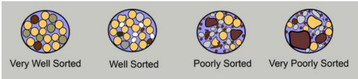
Figure 3-6: Sorting of grains. [23]
