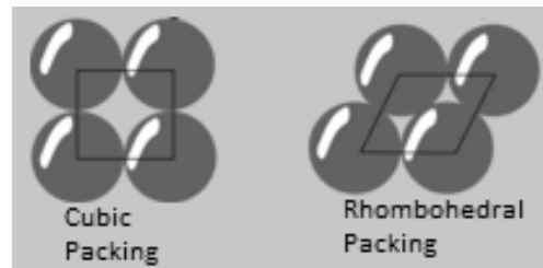
Figure 3-8: Cubic and rhombohedral packing of spheres. [23]
