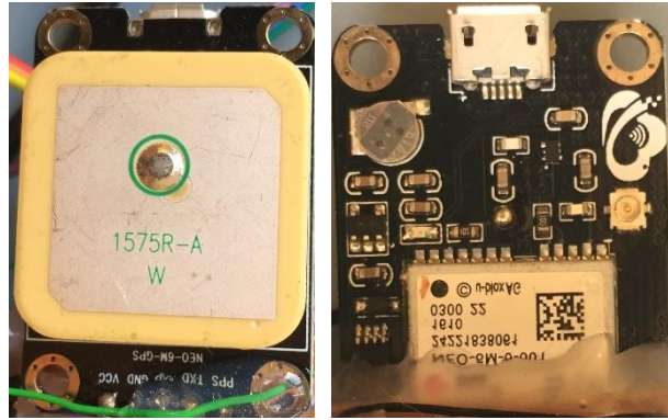
Figure 4.5 The real product of UBLOX 6M GPS module
