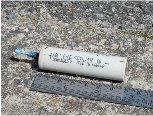
Figure 2. Picture of an 18650 Li-ion battery after a rupture test.
