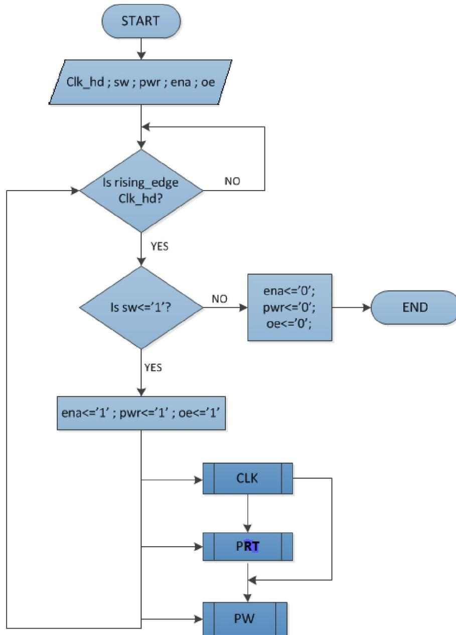
Figure 25: The flow char of the top level process MAIN in the design.
