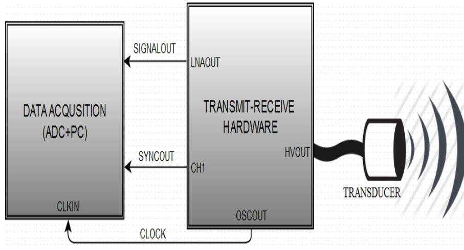
Figure 5: The overall system block diagram.
