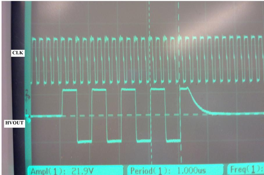
Figure 34: The AC coupled local oscillation output (top) from PCB4(Figure 6) and the HVOUT (bottom) from PCB1(Figure 6).
