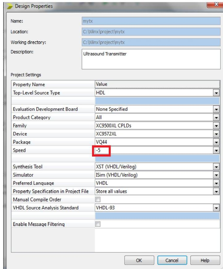
Figure 22: The design properties configuration of the CPLD chip in ISE design suite.
