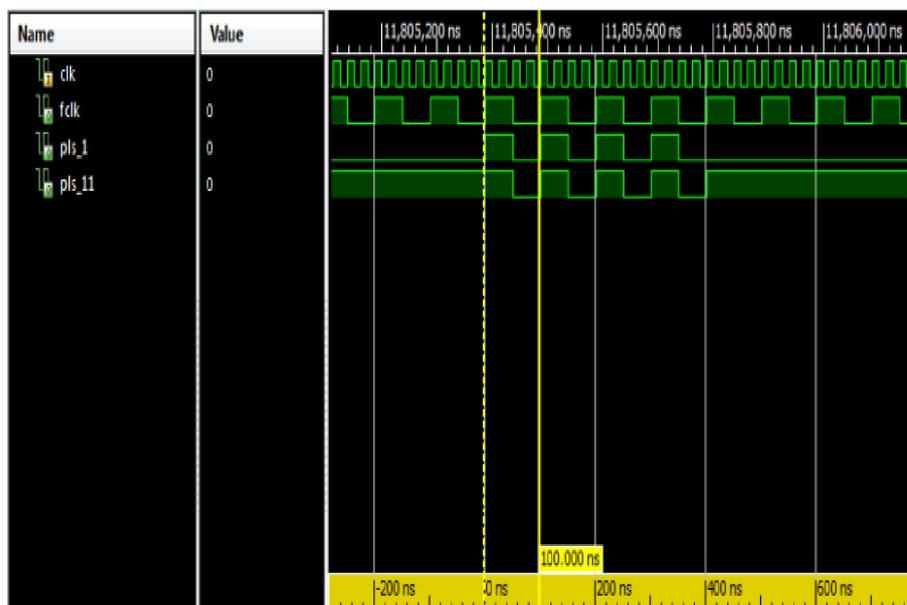
Figure 30: The behaviour simulation of the beamformer for the for the four pulse cycle.
