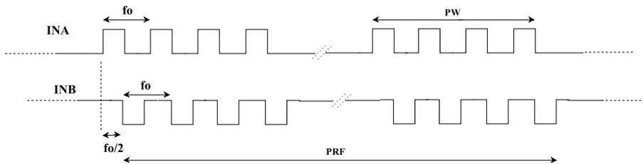
Figure 9: The outputs INA and INB from the CPLD.
