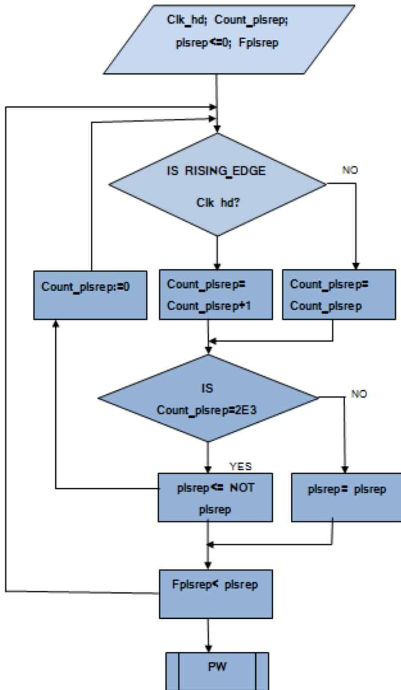
Figure 27: The flow chart for pulse repetition rate PRT module in the design.
