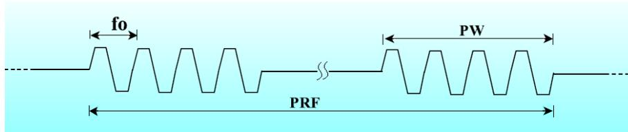
Figure 20: The output waveform of the transmitter.
