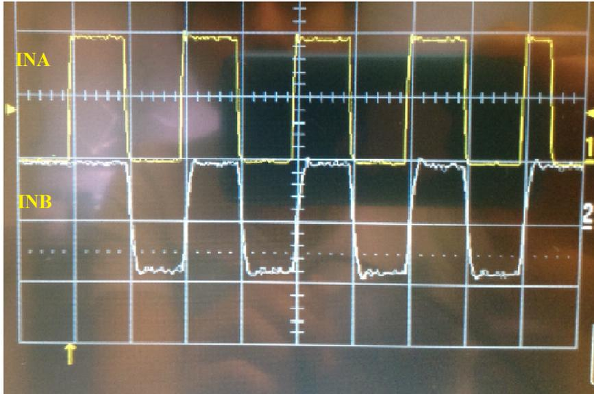
Figure 32: The output from CPLD for 4 pulse cycle.
