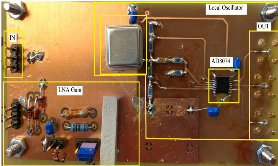
Figure 14: The oscillator and gain board.
