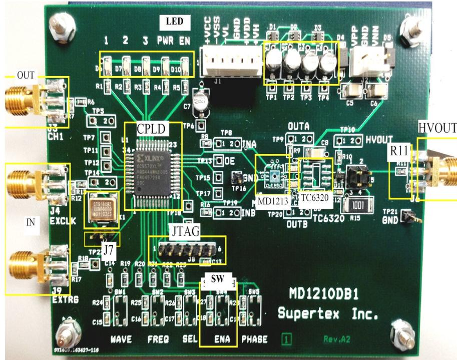
Figure 7: The MD1210DB transmitter board [1].
