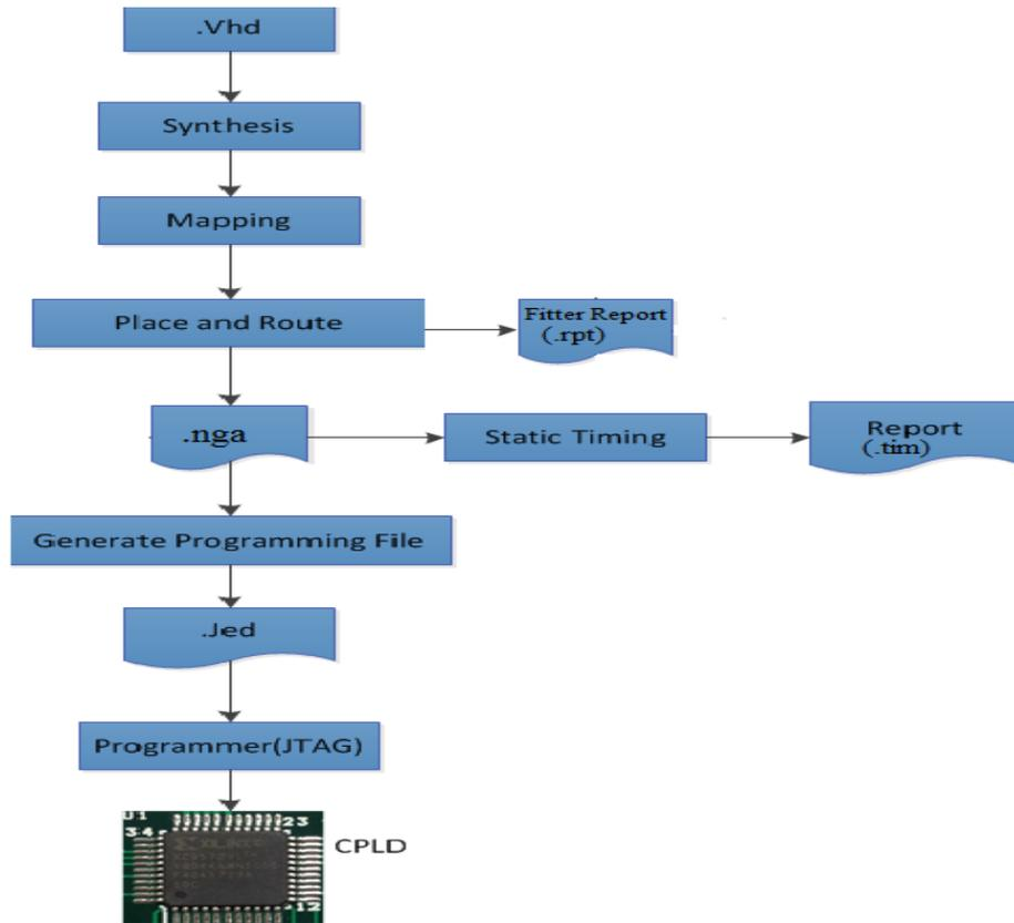
Figure 21: The VHDL design flow in ISE design suite.
