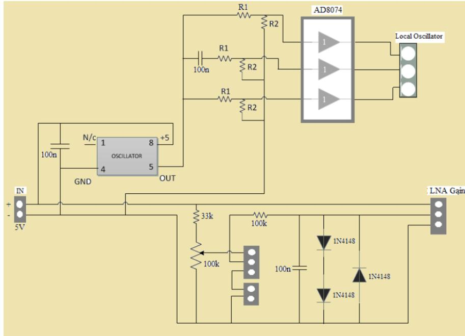
Figure 15: The oscillator and gain board circuit diagram.
