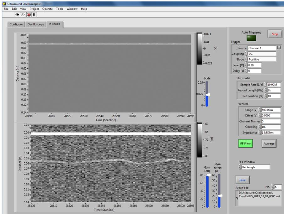
Figure 36: M-mode ultrasound investigation for 1 MHz single element transducer in water.
