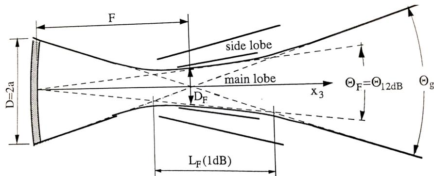
Figure 4: Ultrasound beam focusing from spherical shell disc ( $D$  is aperture,  $a$  is wavelength of the ultrasound) [5].
