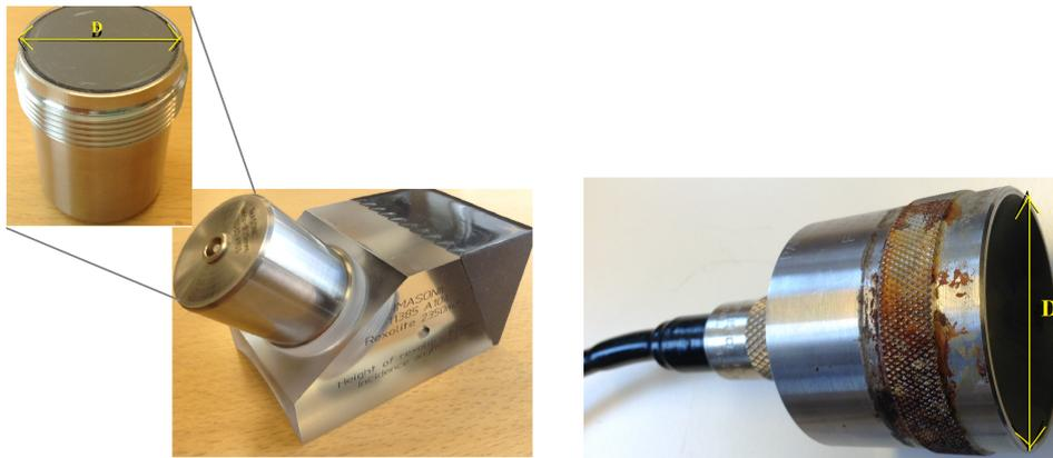
Figure 18: Single element ultrasound transducers.
