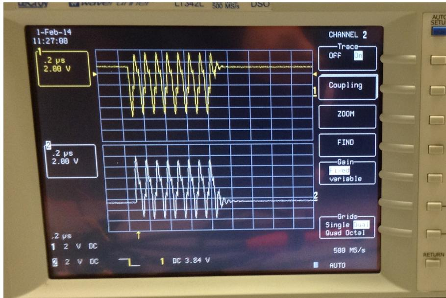
Figure 33: The output from CPLD for 8 pulse cycle.
