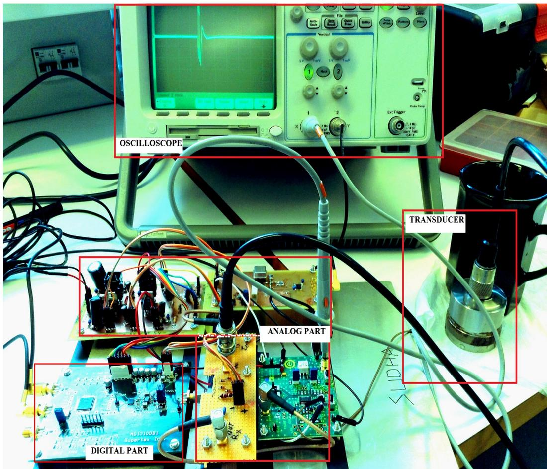
Figure 19: The Ultrasound Test Setup with the designed system.
