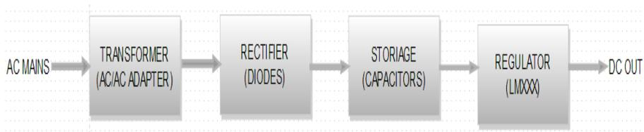
Figure 29: The regulated power supply board block diagram.
