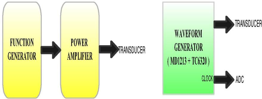
Figure 2: Block diagram of conventional analog function generator (left) and the digital waveform generator (right).
