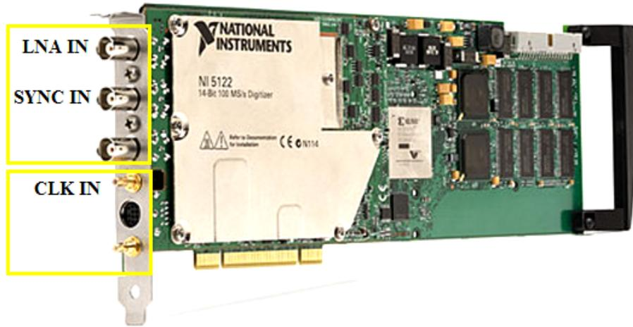
Figure 17: The 14-bit 100MS/s digitizer from National Instruments(NI PCI-5122).[3]
