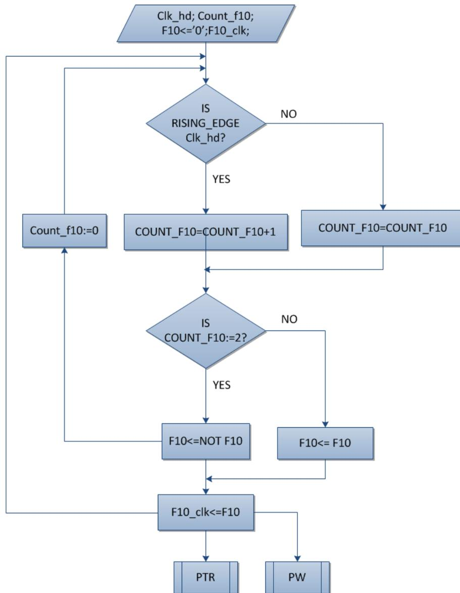
Figure 26: Flow chart of the CLK module use to get the ultrasound frequency in the design.
