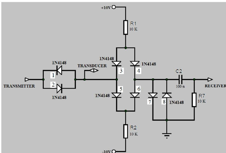
Figure 11: A single channel T/R switch passive circuit.
