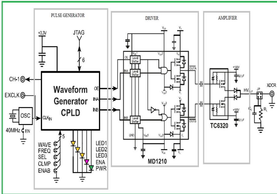
Figure 8: The MD1210DB transmitter board circuit diagram [1].
