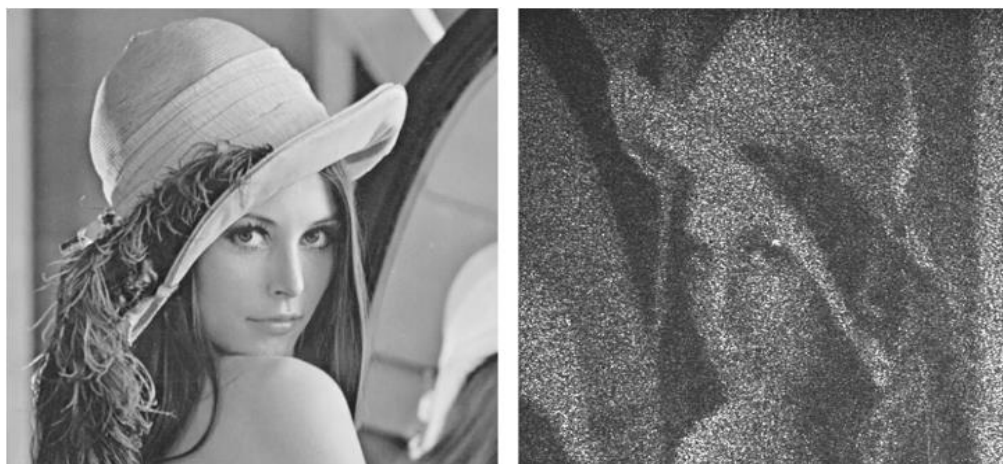
Fig. 3 Speckle free projected image (left) and the image with speckle noise (right).
