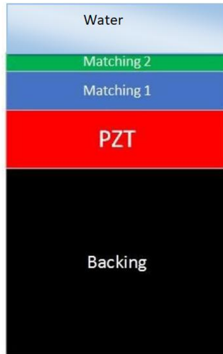
Figure 2.3: A schematic of a typical piezoelectric transducer
