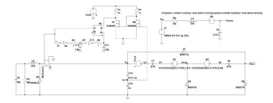
Figure 4.23: The linear-spring doubler circuit connected to a buck converter with controlled electronic switch
