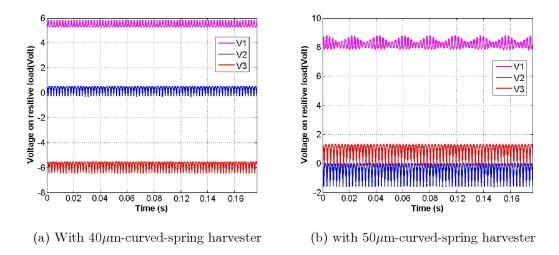
Figure 5.10: The voltage at nodes 1, 2 and 3 of the doubler circuit with  $40\mu$ m- and  $50\mu$ mcurved-spring harvester.
