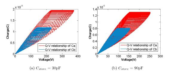
Figure 4.14: Q-V plane contours of two harvesting capacitors of linear-spring doubler
