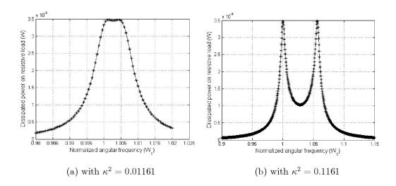
Figure 2.4: Output power peak versus normalized angular frequency under optimal load resistance condition.
