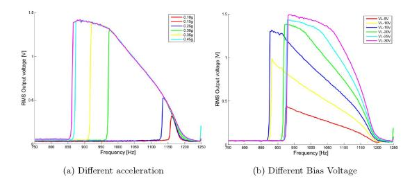
Figure 5.6: The output voltage of  $40\mu$ m curved-spring harvesters with different accelerations a) and bias voltages Ve b).
