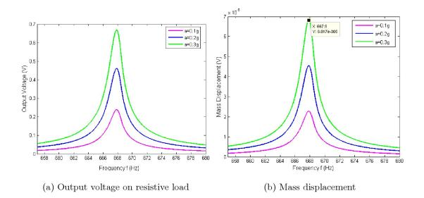
Figure 4.2: Output voltage and mass displacement of a linear-spring harvester with Ve = 5 V when acceleration changes from 0.1 to 0.3 g.
