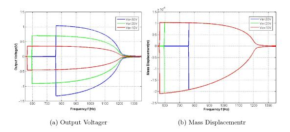
Figure 4.8: Output voltage and mass displacement of a  $50\mu$ m-curved-spring harvester with 0.2 g acceleration in frequency down sweep when Ve = 10, 20 and 30 V.
