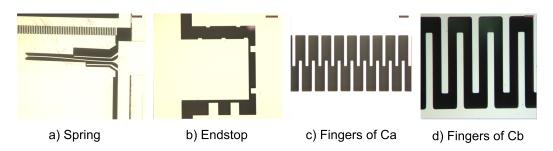
Figure 5.2: The spring, endstop, and fingers of the curved-spring harvester with  $40\mu$ m tip displacement.
