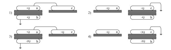
Figure 1.2: The operation of the doubler of charge.
