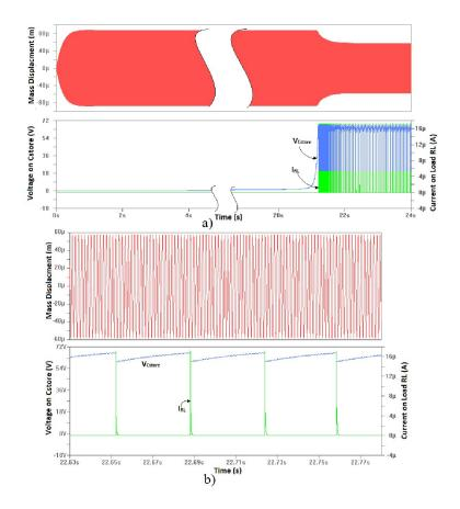
Figure 4.24: Load Current, Voltage on  $C_{store}$  and mass displacement of linear-spring doubler connected to a buck converter with controlled electronic switch, diode BAS716 and 0.25 acceleration) during transient state a) or during steady state b)..
