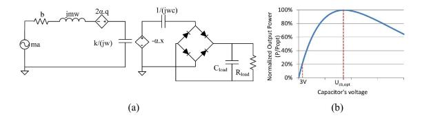
Figure 3.1: (a) Simple passive power converter with diode bridge and (b) optimal output voltage at  $U_{Cb}$  [2].
