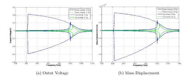
Figure 4.5: Output voltage and mass displacement of a  $40\mu$ m-curved-spring harvester with Ve = 20 V in frequency down sweep when a = 0.1 and 0.3 g.
