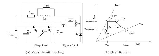
Figure 3.7: An example of combined voltage- and charge-constrained converters [5].
