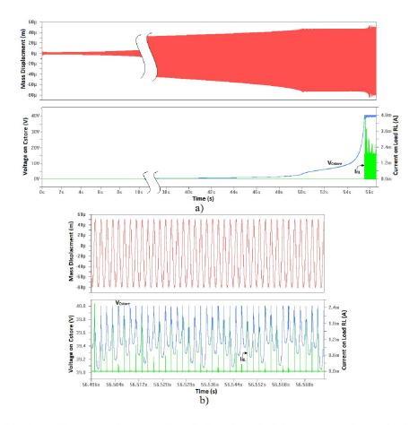
Figure 4.30:  $I_{load}$ ,  $V_{Cstore}$  and  $x_{mass}$  of angled-spring doubler connected to a buck converter with MEMS switch and diode BAS716 during transient state a) or steady state b).
