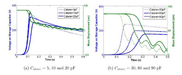
Figure 4.13: Voltage on  $C_{store}$  and mass displacement of linear-spring doubler with different values of storage capacitor  $C_{store}$
