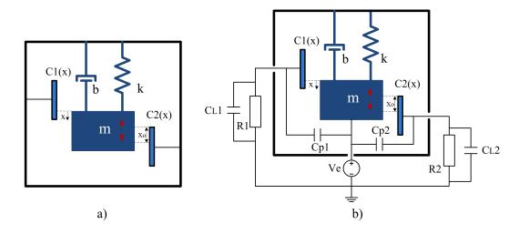
Figure 2.2: In-plane overlap harvesters modesl a) without and b) with resistive load [1].
