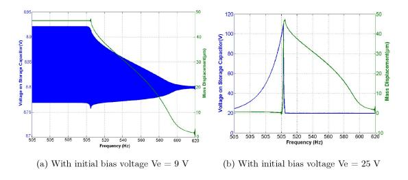
Figure 4.22: Voltage on  $C_{store}$  and mass displacement of angled-spring doubler with  $C_{store} =$  90 pF and diode BAS716.
