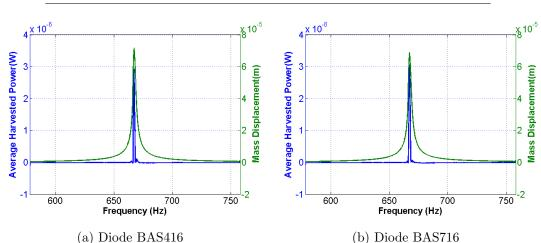
Figure 4.19: A comparison in harvested power and mass displacement of linear-spring doubler with two different diodes at Ve = 60 V, a = 0.38 g
