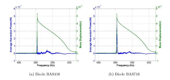
Figure 4.20: A comparison in harvested power and mass displacement of angled-spring doubler with two different diodes at Ve = 30V, a = 0.25 g
