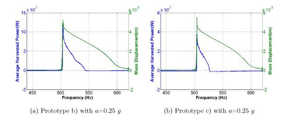
Figure 4.12: A comparison in harvested power of angled-spring doubler between two different asymmetrical structures
