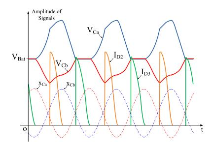
Figure 3.9: Voltage, charge and displacement waveforms on harvesting capacitors in doubler operation.
