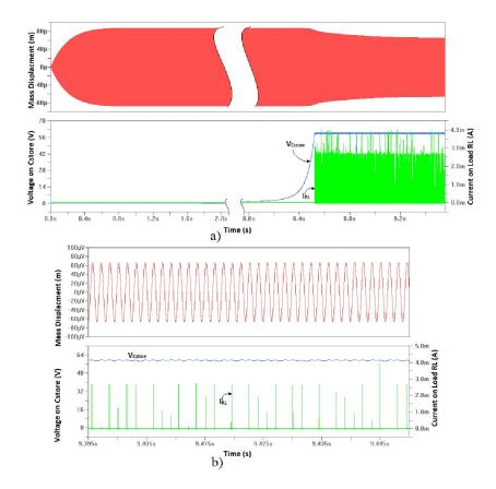
Figure 4.28: Load Current, Voltage on  $C_{store}$  and mass displacement of linear-spring doubler connected to a buck converter with MEMS switch and diode BAS716 during transient state a) or during steady state b).
