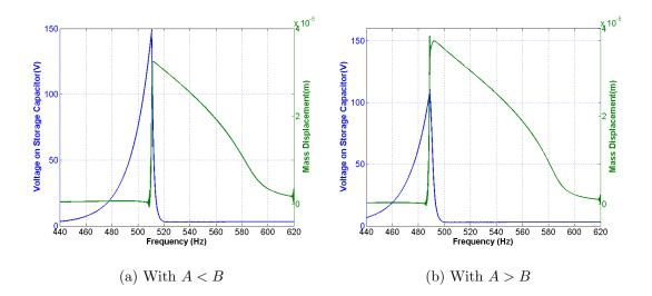
Figure 4.15: A comparison in voltage on  $C_{store}$  and mass displacement of two angled-spring prototypes with  $C_{store} = 90 \text{ pF}$
