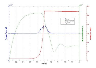
Figure 4.21: Voltage on  $C_{store}$ , output power and mass displacement of linear-spring doubler with  $C_{store} = 90$  pF and diode BAS716
