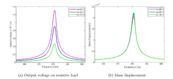
Figure 4.1: Output voltage and mass displacement of a linear-spring harvester with 0.1 g acceleration when Ve =10, 20 and 30 V.
