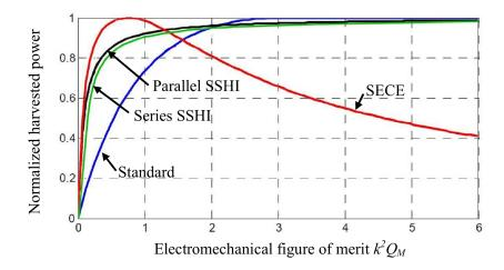
Figure 3.4: Harvested powers of different power converters as a function of the electromechanical figure of merit [2].
