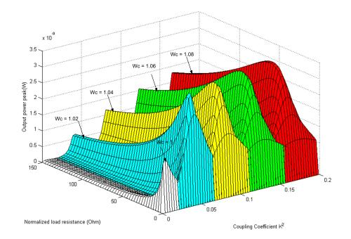
Figure 2.6: Output power performance versus angular frequency and load resistance with different normalized vibration frequency.
