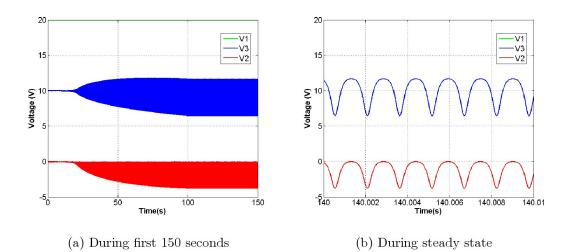
Figure 4.17: Voltage at nodes 1,2 and 3 of the doubler with 50  $\mu$ m curved spring.
