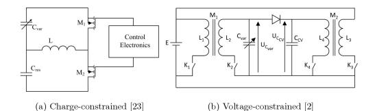
Figure 3.6: Two types of switched electrostatic harvesting system.
