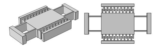
Figure 2.1: The in-plane overlap harvester with linear spring.
