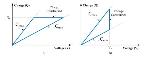
Figure 3.5: a) Charge-constrained conversion cycle and b) voltage-constrained conversion cycle.
