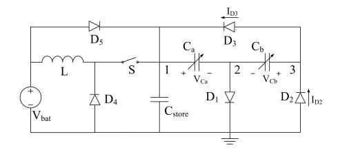
Figure 3.13: The doubler of charge with a buck converter.
