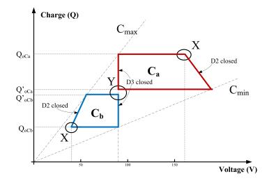
Figure 3.12: Q and V diagram of harvesting capcitors with nonlinear spring.
