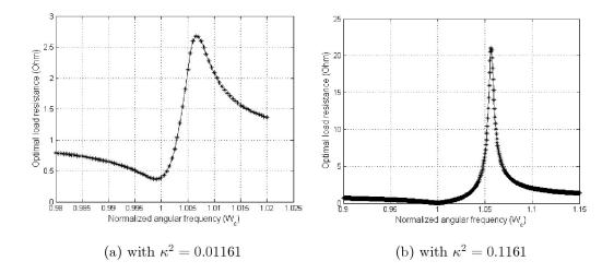
Figure 2.5: Relationship between optimal normalized load resistance and angular frequency.
