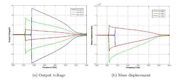
Figure 4.4: Output voltage and mass displacement of a angled-spring harvester with 0.2 g acceleration when Ve =10, 30 and 60 V.
