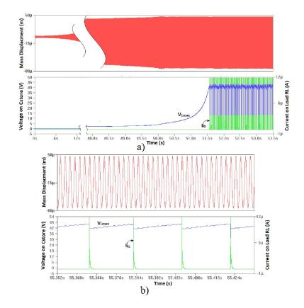
Figure 4.26: Load Current, Voltage on  $C_{store}$  and mass displacement angled-spring doubler connected to a buck converter with controlled electronic switch during transient state a) or during steady state b).
