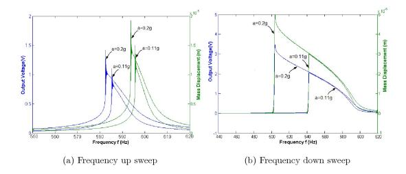
Figure 4.3: Output voltage and mass displacement of a angled-spring harvester with Ve = 30 V when a = 0.11 and 0.2 g.
