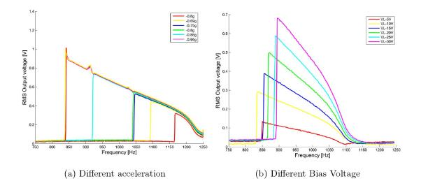
Figure 5.7: The output voltage of  $40\mu$ m curved-spring harvesters with different accelerations a) and bias voltages Ve b).
