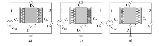
Figure 4.10: Symmetrical and asymmetrical prototypes of the doubler circuits
