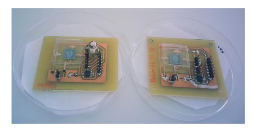
Figure 5.4: The PCBs with doubler circuits and curved-spring harvesters
