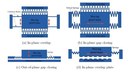
Figure 1.1: Four popular topologies of electrostatic energy harvesting.
