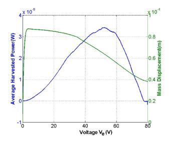
Figure 4.9: Output power and mass displacement as functions of bias voltage Ve.
