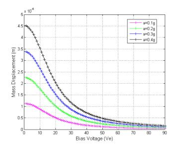
Figure 2.7: Mass displacement versus bias voltage Ve with different acceleration values.
