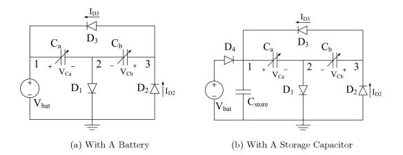
Figure 3.8: The doubler of charge topologies.
