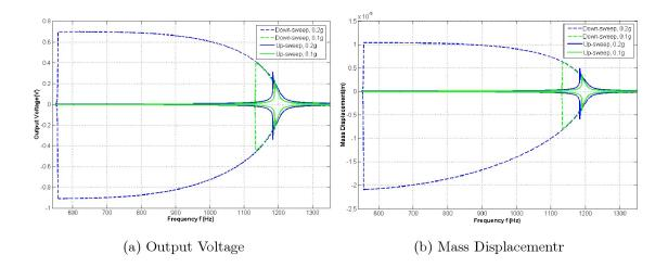
Figure 4.7: Output voltage and mass displacement of a  $50\mu$ m-curved-spring harvester with Ve = 20 V in frequency down sweep when a = 0.1 and 0.2 g.
