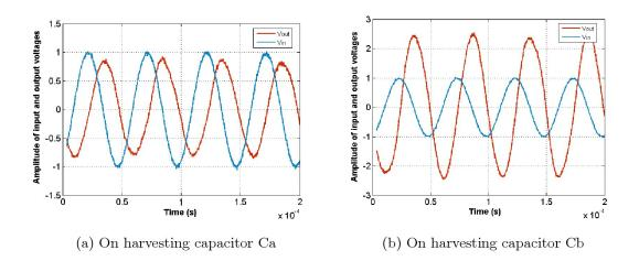
Figure 5.13: Output and input voltage of the measurement circuit when measuring the  $50\mu$ m-curved-spring doubler.
