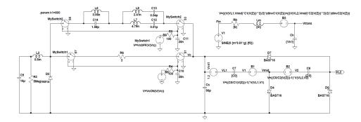
Figure 4.27: The linear-spring doubler circuit connected to a buck converter with MEMS switch
