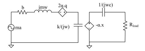
Figure 2.3: Equivalent circuit of the linear harvesting system with resistive load.
