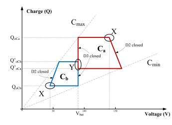
Figure 3.10: Voltage and charge diagram of harvesting capacitors with linear spring.
