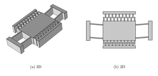
Figure 2.8: Curved-spring harvester.
