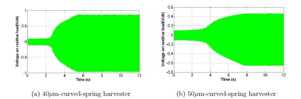
Figure 5.9: The output voltage of the  $40\mu$ m- and  $50\mu$ m-curved-spring harvesters with vibration frequency sweep.
