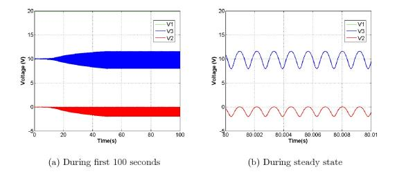
Figure 4.16: Voltage at nodes 1,2 and 3 of the doubler with 40  $\mu$ m curved spring.
