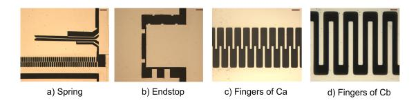
Figure 5.3: The spring, endstop, and fingers of the curved-spring harvester with 50  $\mu$ m tip displacement.
