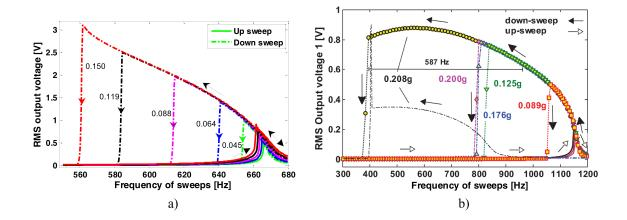
Figure 2.11: Output voltage in down/up sweep of energy harvester with a) angled spring or b) curved spring.
