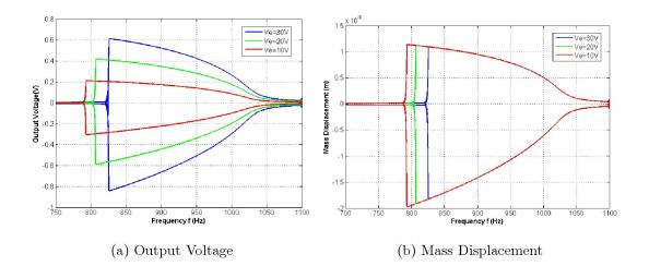
Figure 4.6: Output voltage and mass displacement of a  $40\mu$ m-curved-spring harvester with 0.3 g acceleration in frequency down sweep when Ve = 10, 20 and 30 V.
