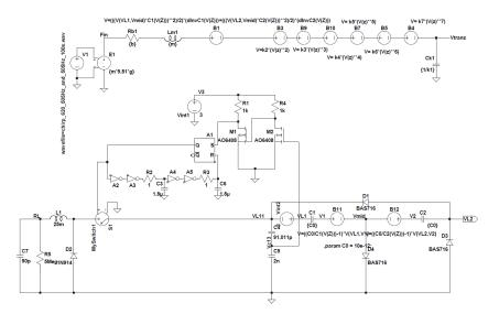
Figure 4.25: The angled-spring doubler circuit connected to a buck converter with controlled electronic switch
