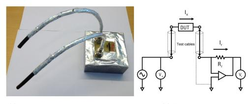
(a) Parasitic capacitance measurement box
