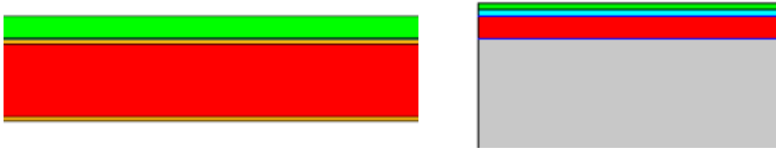
Figure 3.7 – Enlarged section of COMSOL model of the mid-frequency transducer (left) and high-frequency transducer (right). Mid-frequency transducer is modeled with piezoelectric element (red domain) with electrodes on both sides, a bond line (not visible) and a matching layer. High frequency transducer is modeled with a piezoelectric element with electrodes on both sides, two matching layers and a backing layer.
