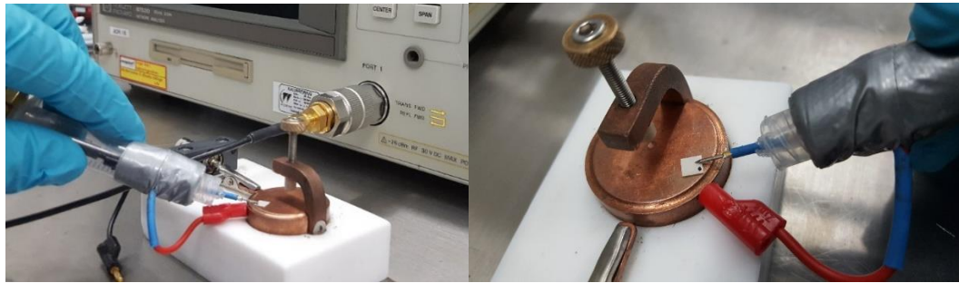
Figure 3.11 – Electrical impedance measurement setup for characterizing mid-frequency transducers. The network analyzer was calibrated for the needle probe shown in the figure. The figure demonstrates how the piezoelectric element alone was measured. The copper chuck was also calibrated for in this case.
