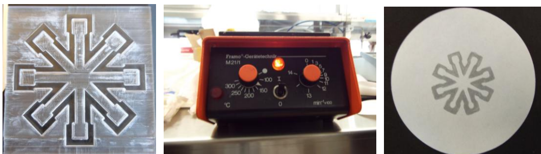
Figure 4.7 Realization the fabrication process in the lab. a) the module fabricated by the laser cutting machine; b) the baker; c) the final made product.
