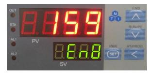
Fig. 2.6 Temperature controller panel
