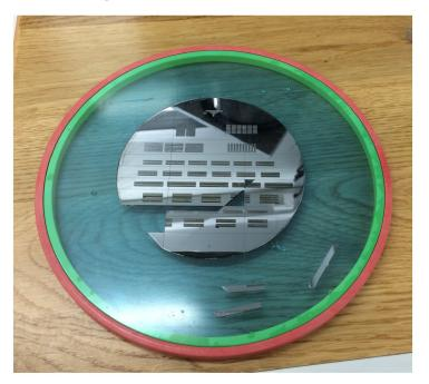
Fig. 5.6 wafer after finishing SU-8 process
