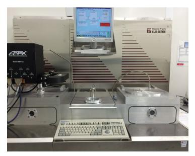
Fig. 2.9 Reactive Ion Etcher
