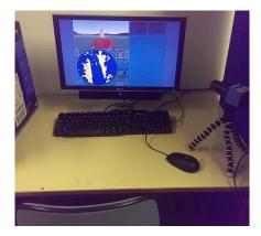
*Figure 9*. Workstation of the Master equiped with a RADAR, visual lookout, a keyboard and a mouse.
