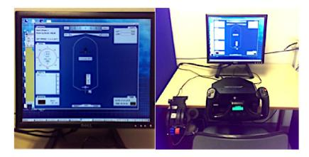
*Figure 11*. Workstation of the Helmsman equipped with conning display, a steering wheel and speed throttle.
