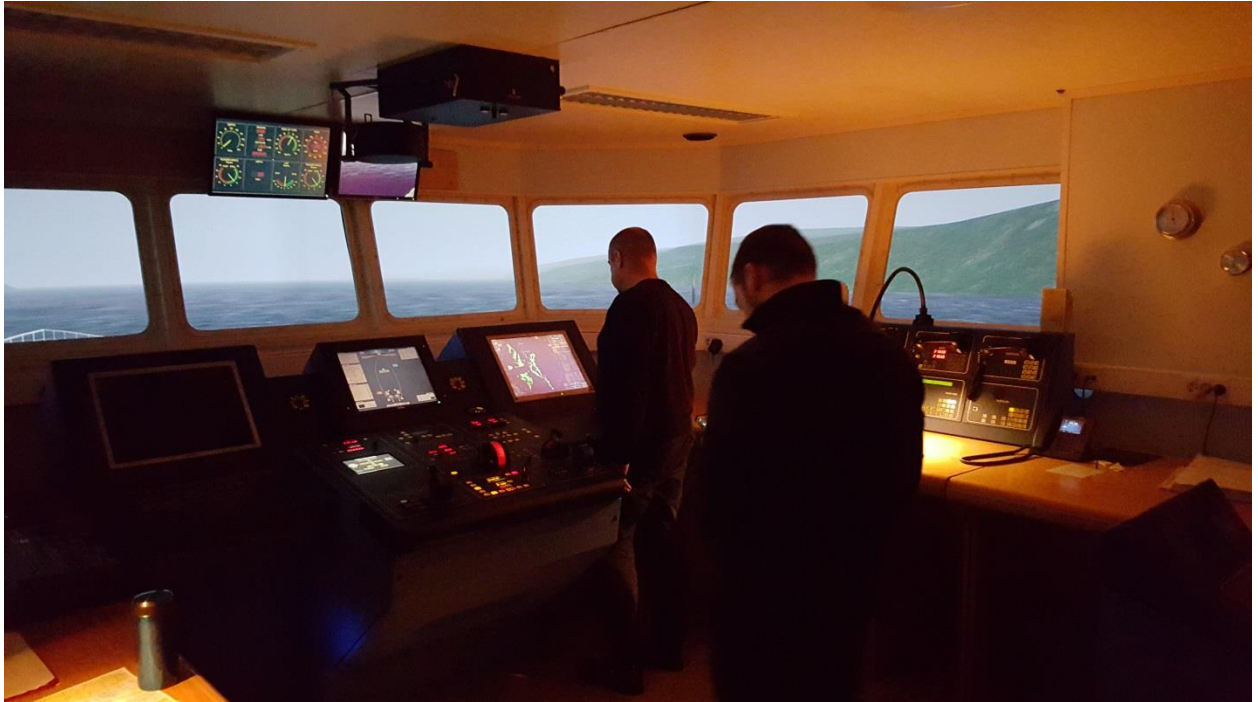
Figure 1: “Horten” Navigation Simulator at USN - Kongsberg Bridge Line 10 simulator (upgraded to K-Bridge software) with a 225° forward view (copyright author).
