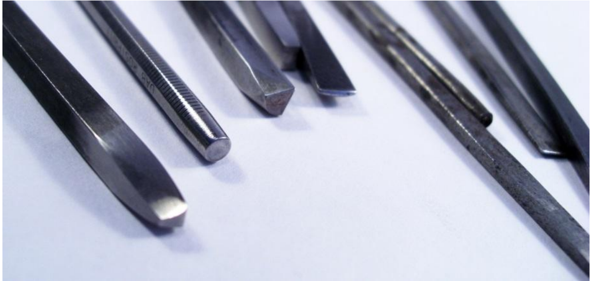
Fig.18 Selection of the modern punches which was using for making relief on the bracteates.
