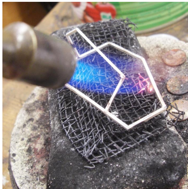
Fig. 63 The process of soldering
