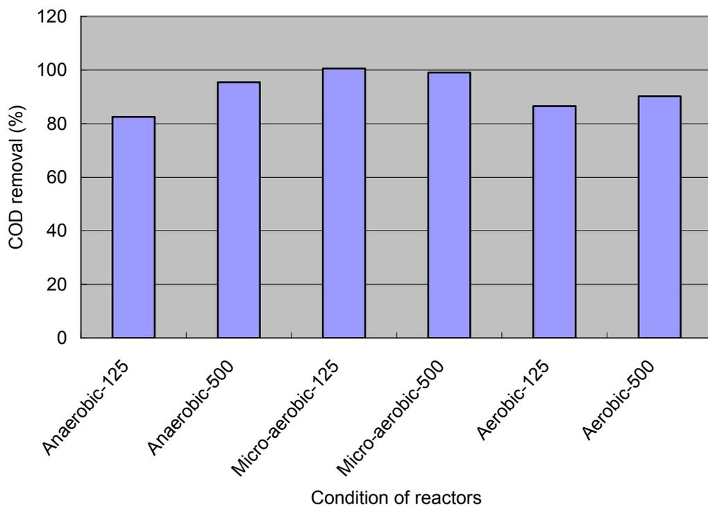
**Fig. 12. COD removal by the 21<sup>st</sup> day of the syringe experiment in reactors under 6 different conditions.**
