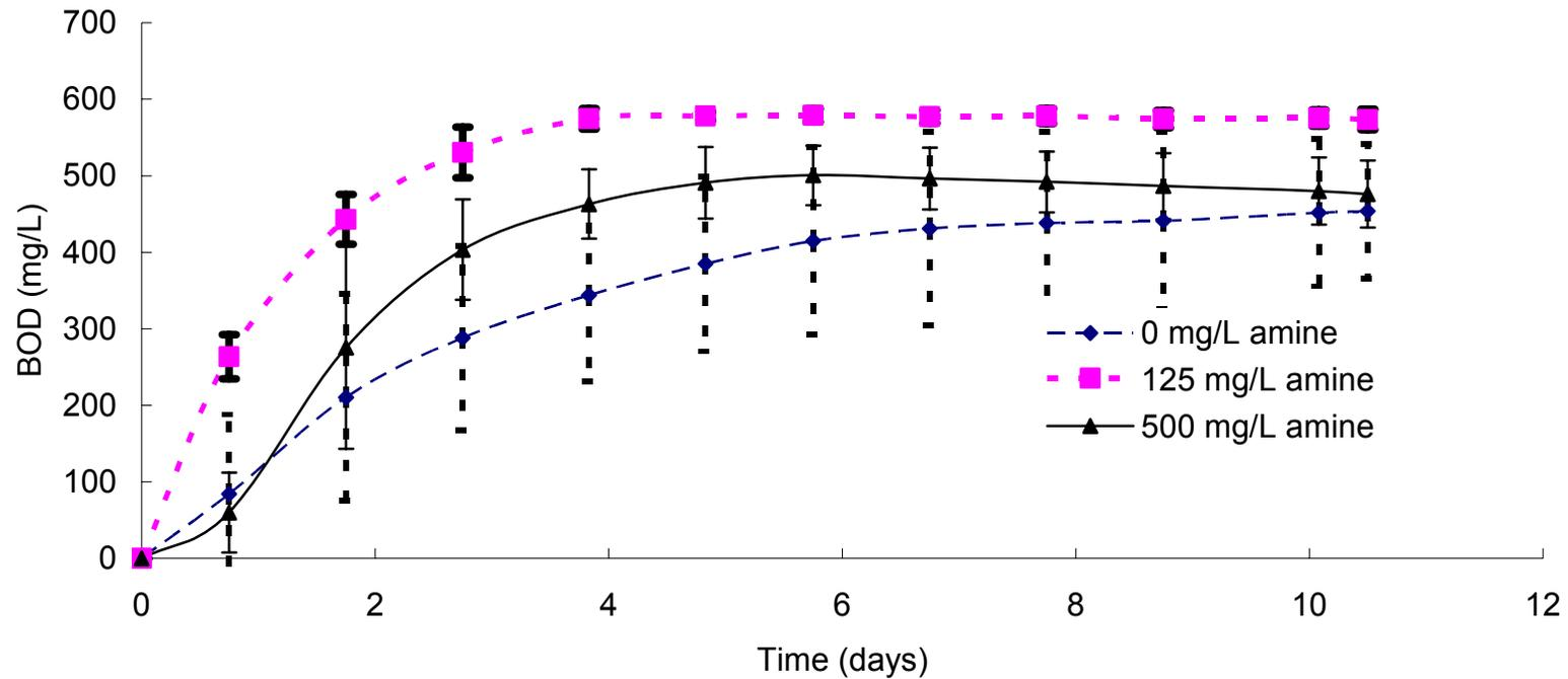
**Fig. 2. Results of BOD test series 1 showing consumed oxygen as average of two parallels for 3 amine levels, as a function of time.**
