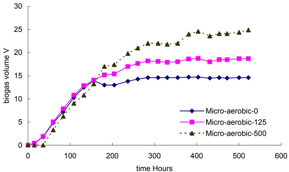
**Fig. 9. Biogas production in micro-aerobic reactors showing accumulated biogas produced as average of parallels for 3 amine levels, as a function of time.**
