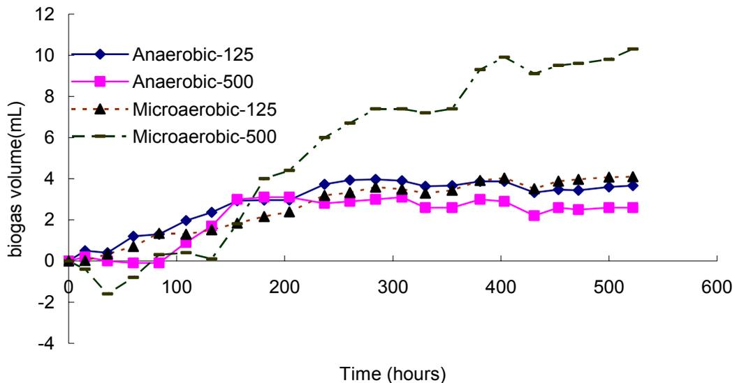
**Fig. 13. Net biogas production showing net biogas production as average of parallels in two anaerobic and two micro-aerobic cases with 2 amine levels of each case, as a function of time.**
