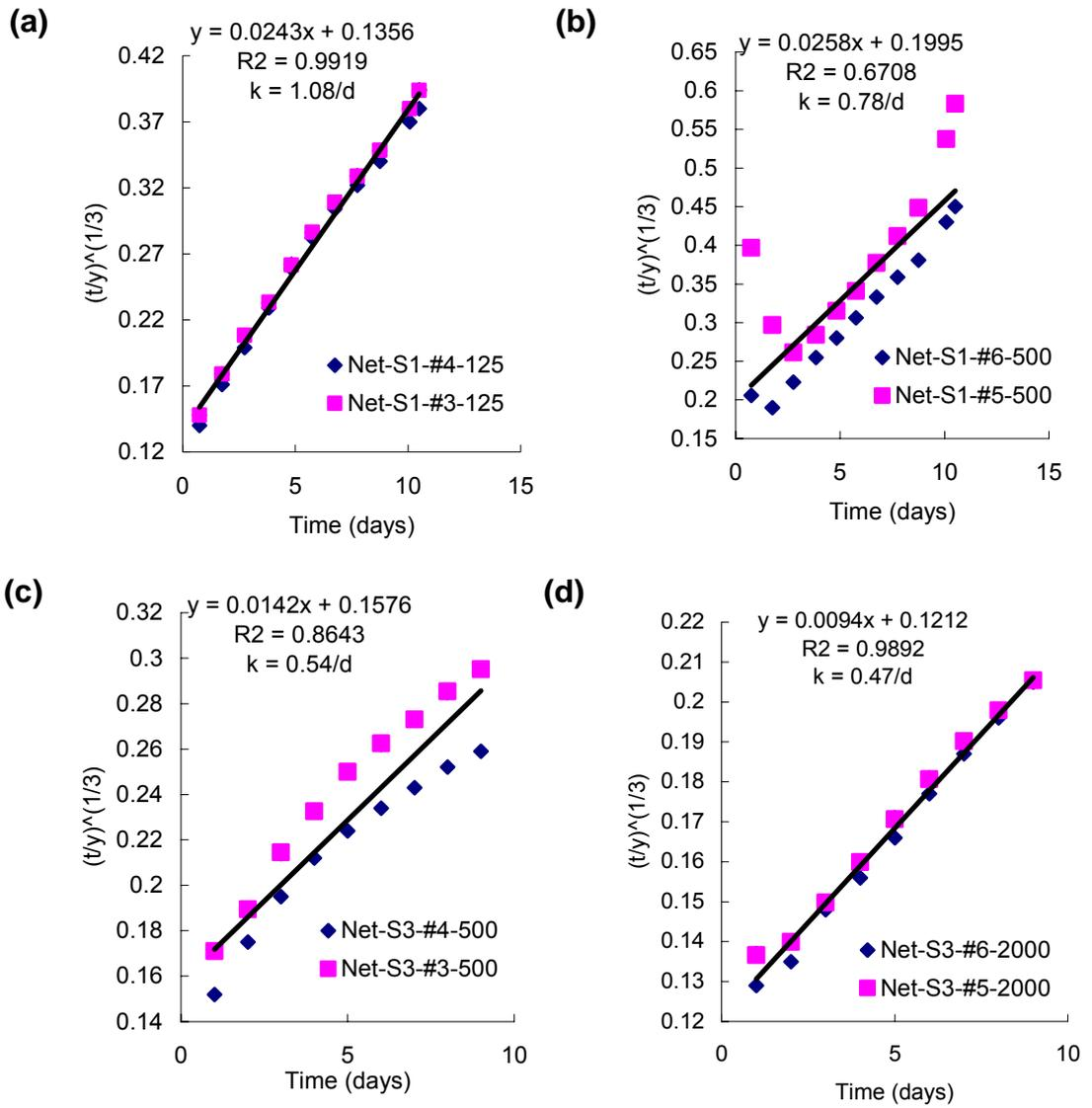
**Fig. 7. Net reaction rate  $k$  and linearization of data for reactors in BOD test series 1 and 3.**
