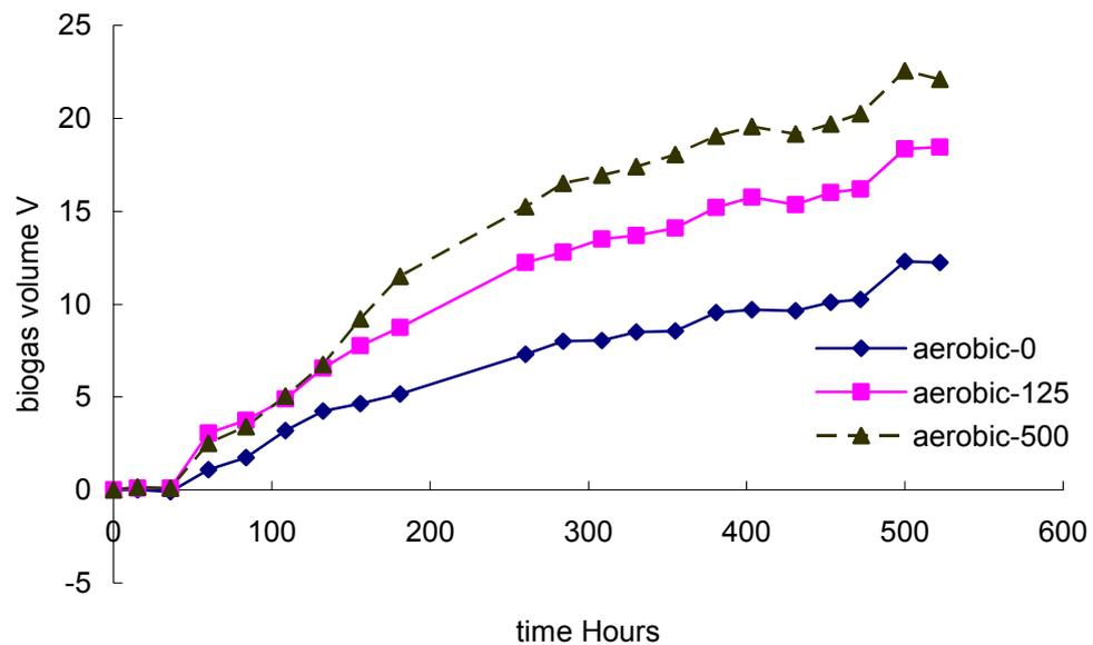
**Fig. 10. Biogas production in aerobic reactors showing accumulated biogas produced as average of parallels for 3 amine levels, as a function of time.**
