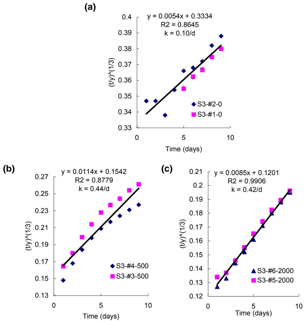
**Fig. 6. First order BOD removal rate  $k$  and linearization of data for reactors with 3 amine levels in BOD test series 3.**
