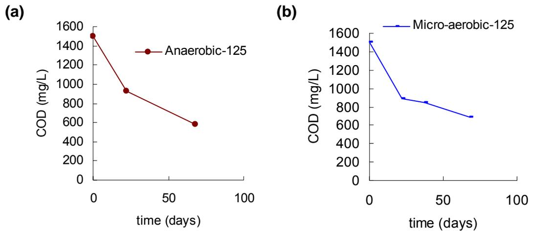
**Fig. 11. COD degradation in anaerobic-125 and micro-anaerobic-125 reactors showing COD degradation as average of parallels, as a function of time.**
