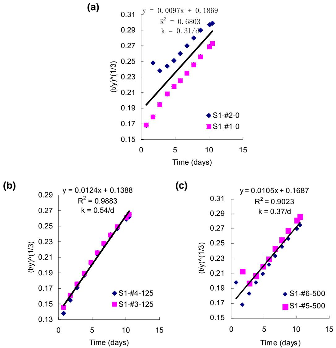
**Fig. 5. First order BOD removal rate  $k$  and linearization of data for reactors with 3 amine levels in BOD test series 1.**
