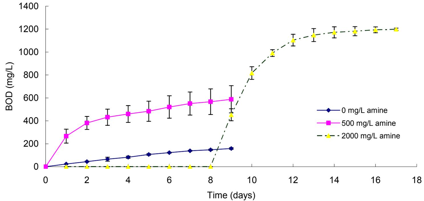
**Fig. 4. Results of BOD test series 3 showing consumed oxygen as average of two parallels for 3 amine levels, as a function of time.**
