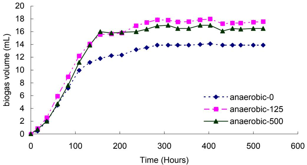
**Fig. 8. Biogas production in anaerobic reactors showing accumulated biogas produced as average of parallels for 3 amine levels, as a function of time.**
