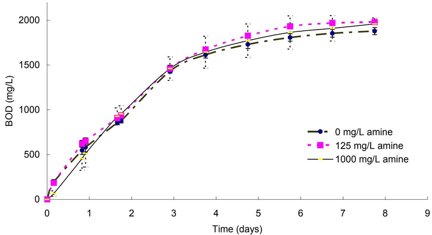
**Fig. 3. Results of BOD test series 2 showing consumed oxygen as average of two parallels for 3 amine levels, as a function of time.**
