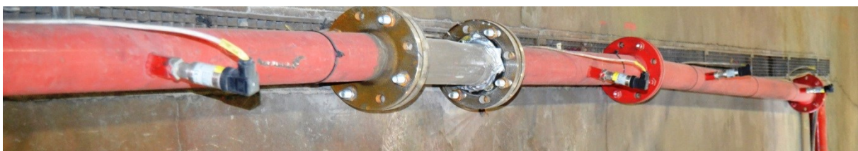
Figure 3-5 Pressure transducers mounted on the pipeline
