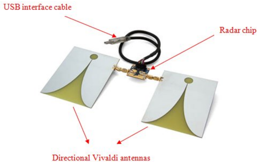
Figure 1.1: Novelda UWB radar system with a pair of directional Vivaldi antennas.
