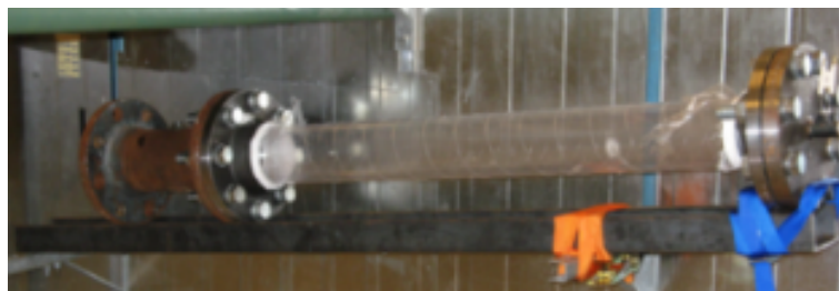
Figure 4.2: Showing the transparent Lexan pipe, steel flanges and steel tail pipe. The obstacle is placed between the tail pipe and the flange.
