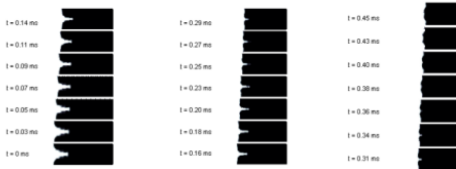
Figure 5.9: Case 2 Mach 1.4 shock wave propagating from reactants to products through the inverted flame. Black part is the products. The sequence shows that flame front changes from inverted back to convex shape.
