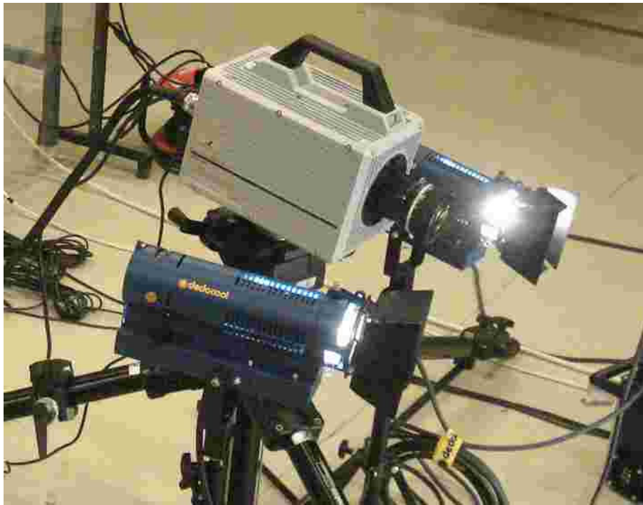
Figure 3-25: A pair of Dedocool lighting lamps for illumination.
