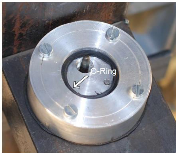
Figure 3-5: O-ring for preventing gas leakage.
