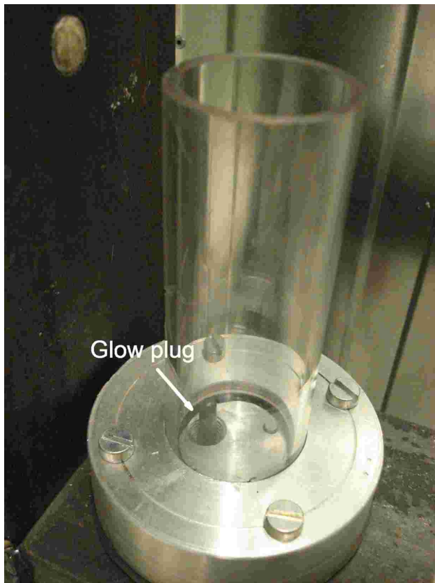
Figure 3-13: Glowing part of the glow plug inside experimental pipe.
