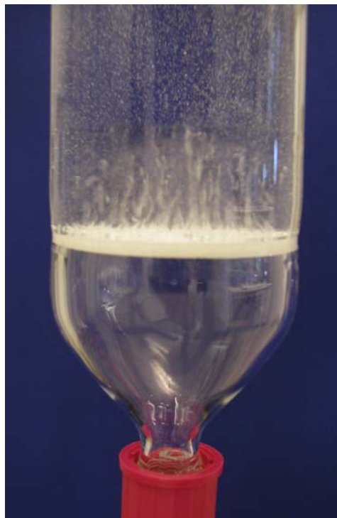
Figure 4 - 2: The phase difference in the MEA solution in the glass column used to load the different MEA solutions. CO 2 is bubbled through the sinter, where large bubbles are observed between the sinter and the phase difference and small bubbles above.
