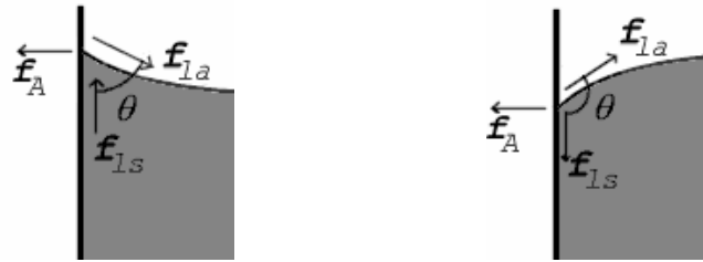
Figure 2 - 2: The forces show a contact angle less than 90^\circ where the meniscus is concave (left) and greater than 90^\circ where the meniscus is convex (right). f_A denotes adhesive (klebrende) force, f_{la} denotes liquid-air (horizontal) force component and f_{ls} denotes liquid-solid (vertical) force component.
