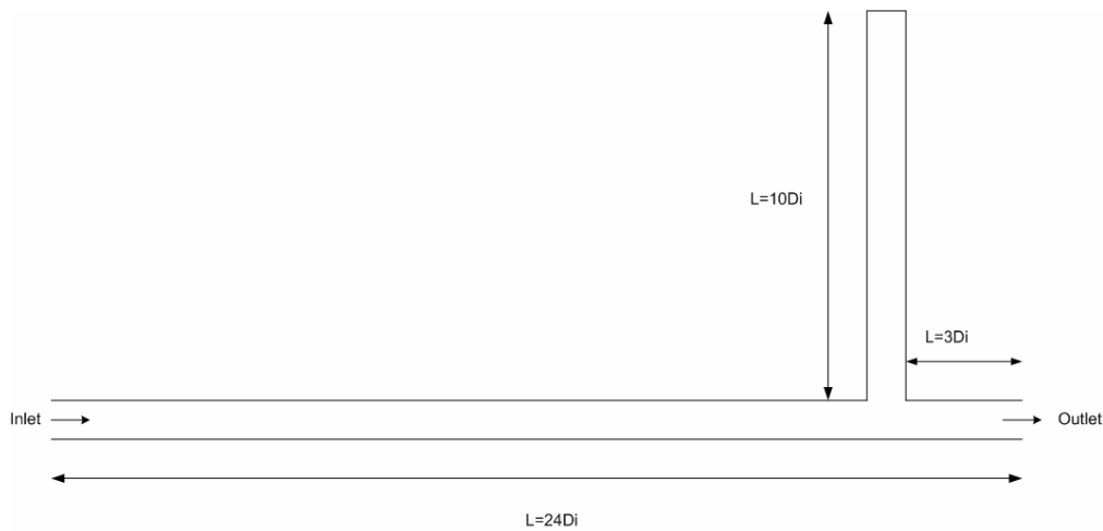
Figure 3-1: Geometry of pipe with branch
