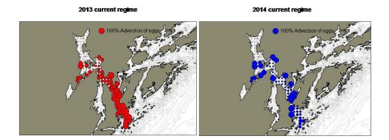
**Figure 16** The amount of particles advected out of the modelled area after drift vary with different current regimes (here 2013 to the left in red and 2014 to the right in blue). The particles were released in a uniform horizontal and vertical distribution in the whole fjord.
