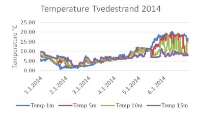
*Figure 21 Measured temperature (from one buoy) in Tvedestrandsfjorden from 17.01 – 01.07 2014 at 4 different depths (1m, 5m, 10m and 15m).*
