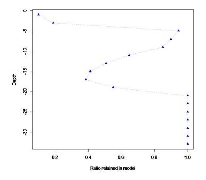
**Figure 15** The ratio of particles retained in the modelled area (fjord) after drift vary at different depths. The particles were released in a uniform geographic distribution and evenly distributed at all depths. The model is based on environmental conditions in March and April 2014 in Tvedestrandsfjorden.
