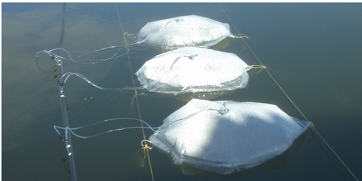
Figure 6 Low cost photobioreactors constructed throughout this work. The floatable bioreactors are maintained by a rope system and the air-supply allows a continuous shuffle of the culture.
