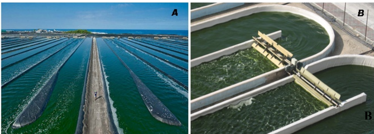
Figure 1. Open pond systems used nowadays by different companies for large-scale production of microalgae: A) Cyanotech Corporation, USA; B) Seabiotic, Israel
