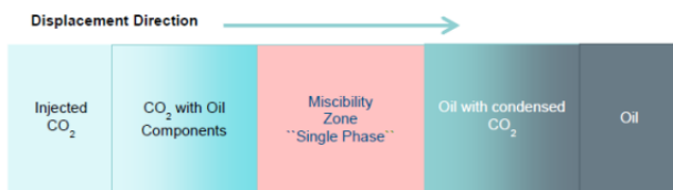
Figure 2. Illustration of the zones that develop in miscible CO 2 flooding (Steve Whittaker 2013)
