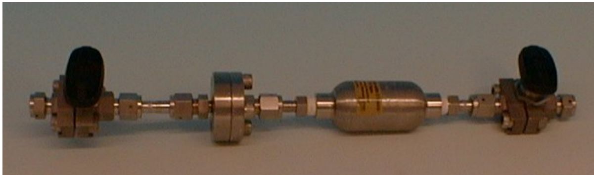
Figure 5.4: Membrane cell for permeability measurements with a gas tank of a volume 0.05 dm 3 (upstream side).
