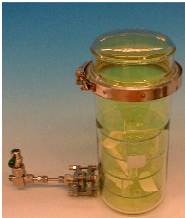
Figure 5.9: Glass chamber used for durability tests of polymer samples.
