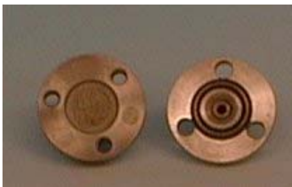
Figure 5.4: Membrane cell for permeability measurements with a gas tank of a volume 0.05 dm 3 (upstream side).
