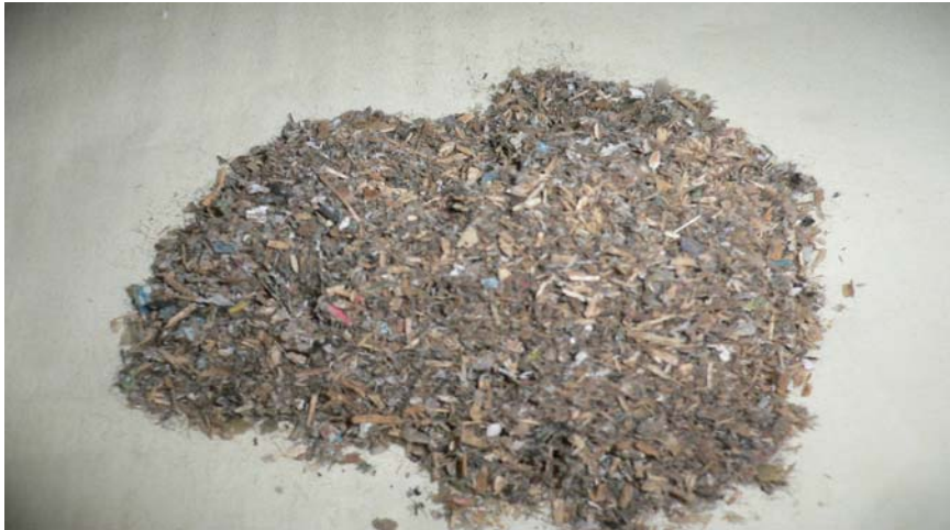
Fig. 1. Pre-dried and shredded Refuse Derived Fuel sample.
