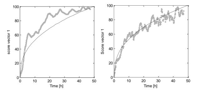
Fig. 5. Principal component analysis score 1 for two independent data sets. The two figures show the growth of the wax deposits in the pipeline for their respective experiments. The nature of the curves show that the wax deposition thickness increases with time. The difference between the wax growths in these two figures can be associated with the temperature difference and the oil density
