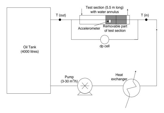
Fig. 1. Experimental wax deposition test rig [16]
