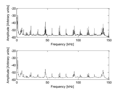
Fig. 4. Acoustic spectrum before pre-processing (top) and after pre-processing (bottom). A moving average of 366 Hz frequency was computed to smooth each acoustic spectrum
