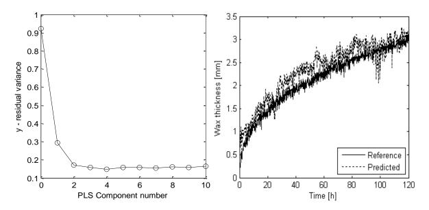
Fig. 7. Left: Explained validation variance plot. 2 PLS components can be considered to be the optimum for model calibration. Right: Predicted and reference time series plot for online prediction of the wax deposition thickness during the 5 days experimental period. The model was validated with an independent data set (Test set validation).
