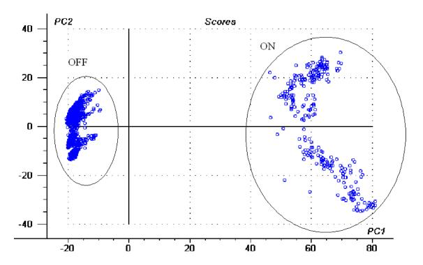
Fig. 6. Principal component analysis scores 1 & 2 to illustrate the heater being either on or off. From this figure, two clear groups can be seen and more data was acquired when the heater was off
