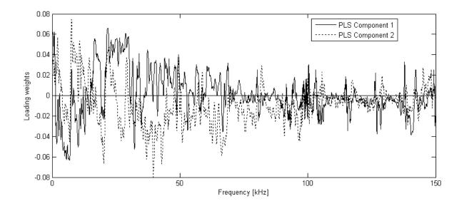
Fig. 8. Loadings weight plot showing the 1<sup>st</sup> and 2<sup>nd</sup> PLS components. This plots shows that all frequencies can be considered to be important for model calibration even though frequencies less than 70 kHz (left half) were considered to be more important.
