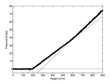
Fig. 3. Application of ordinary least square regression for determining the gas/liquid and oil/water interface levels in a gravity separator considering only downward pressure profile.
