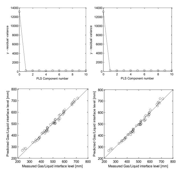
Fig. 4. Liquid level estimation comparison between simulated and experimental data sets. Left: Simulated data, Right: Experimental data, Upper: Residual validation variance plot, Lower: Predicted vs. measured plot.
