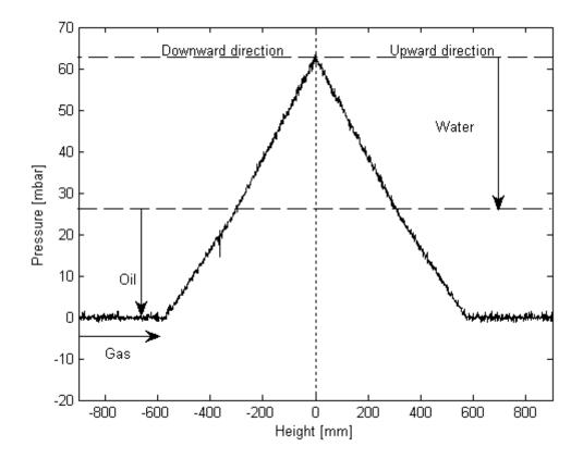
Fig. 2. Pressure profile for a complete cycle of movement of the pressure sensor in the vertical gravity separator
