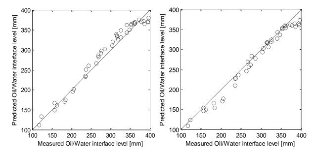
Fig. 6. Comparing the Oil/Water level models predictive properties for the simulated and experimental data sets. The predicted vs. measured plots are shown as an aid for this comparison. Left: Simulated data set. Right: Experimental data set
