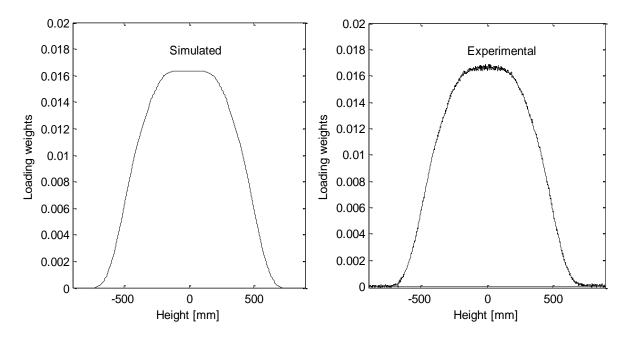
Fig. 5. Comparing the loading weight plots for both simulated and experimental data for PLS component 1. The two plots shows identical profiles but the experimental data also includes some measurement noise which can be observed also in the loading weights.
