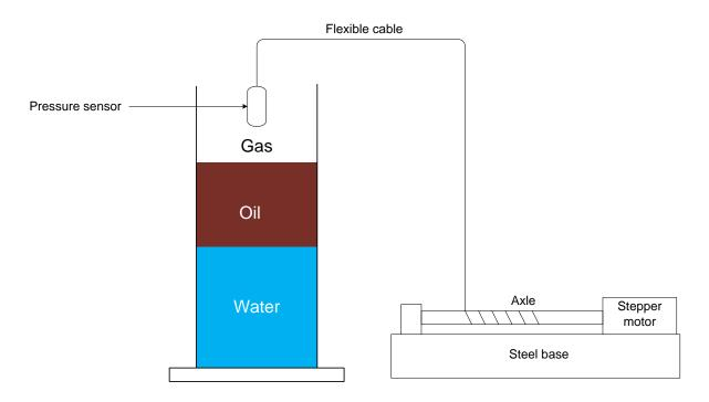
Fig. 1. Experimental test facility with a stepper motor for traversing the pressure sensor from the top to the bottom of the separator and in a reverse cycle for each experimental run
