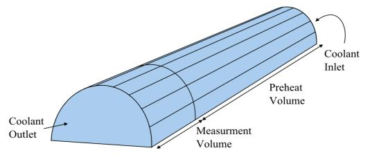
Figure 2 The fluid dynamic geometry. The length of the preheat volume is shortened in this illustration.
