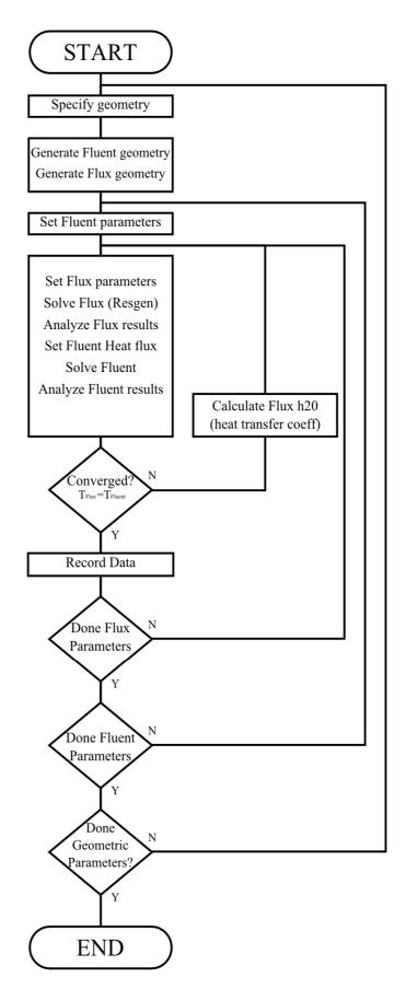
Figure 5 Flow sheet of the solving process.
