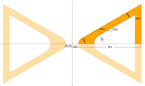
Figure 6 Geometry for investigation of effect of corner inner radius. (**tri** – Tube Radius Inner, **tro** – Tube Radius Outer, **twa** – Tube Wall Angle, **twt** – Tube Width, **tsx** – Tube Size X-direction, and **tds** – Tube distance to vertical Symmetry line.
