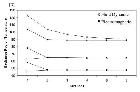
Figure 4 Iteration. Temperature of three different exchange regions in the electromagnetic and in the fluid dynamic domain converging.
