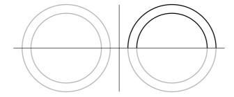
Figure 1 2D plane-symetric geometry with horizontal and vertical symmetry lines. Parts removed from the computational domain by the symmetries are greyed.
