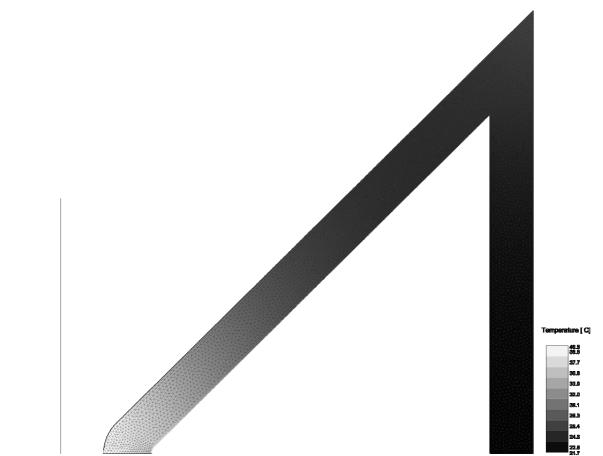
Figure 7 Temperature of the coil cross section when wall angle,  $\mathbf{twa} = 45^{\circ}$  and the radius of the inner corner,  $\mathbf{tri} = 0.25$  mm.
