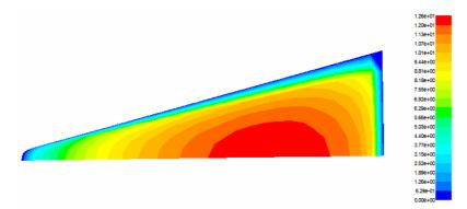
Figure 9 Velocity inside the coil cross section when wall angle,  $twa = 15^{\circ}$  and the radius of the inner corner, tri = 0.25 mm. Coolant velocity in = 10m/s.
