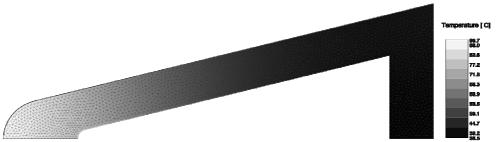
Figure 8 Temperature of the coil cross section when wall angle,  $\mathbf{twa} = 15^{\circ}$  and the radius of the inner corner,  $\mathbf{tri} = 0.25$  mm.
