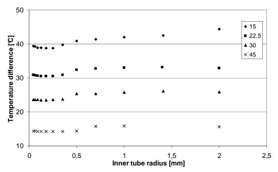
Figure 10 Temperature difference (peak-mean) per tube with different angles.
