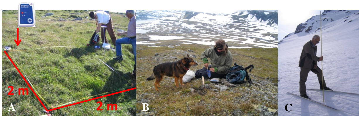
Fig. 3 Field work. A: Study plot of 4m 2 with a temperature data logger to dig down in the upper left corner. B: The author and her field assistant digging out a data logger after one year measurement duration in a study plot on an exposed site at Finse with patchy snow distribution which is typical for mountain areas during spring in the background. C: Snow measurement in the beginning of April.
