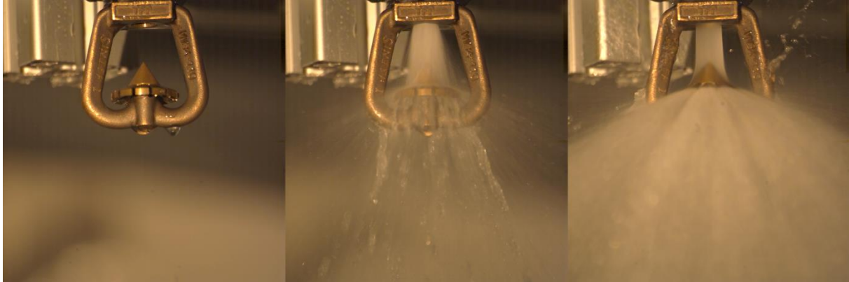
Figure 3.11: Medium velocity nozzle before the water is turned on (left), right after (middle) and when the flow is steady (right). The water pressure was 2.0 bar(g).
