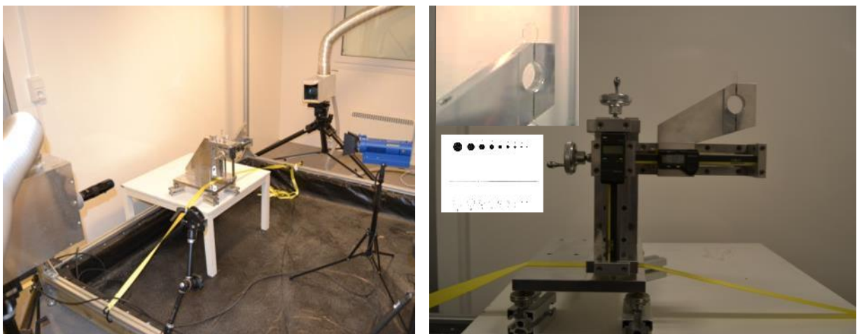
Figure 4.7: Setup with translation screw controlling position of a Patterson globe.
