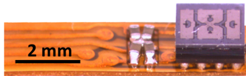
Figure 4.4: Flexible cable/substrate with bonded CMA3000 accelerometer and low pass filter capacitors
