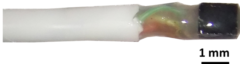
Figure 4.84: The accelerometer device version 2-2 without metal capsule.
