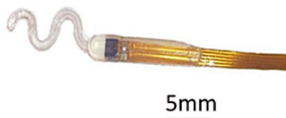
Figure 3.1: The heart muscle accelerometer device (version 1-1) with silicone encapsulation
