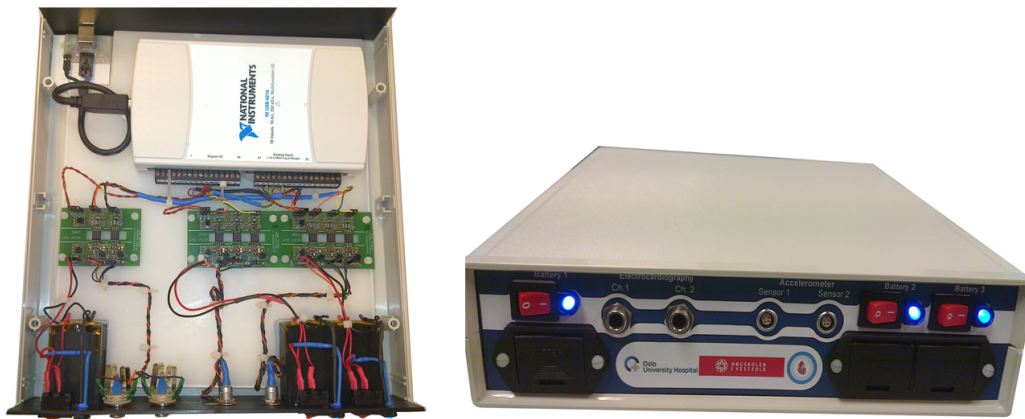
Figure 4.43: The galvanic Isolator used for analogue accelerometer devices (version 1-1, 1-2, and 1-3). The box was built in collaboration with the Intervention centre - Oslo University Hospital and got the approval for internal use. The circuit was designed by Fred-Johan Pettersen (Researcher at Oslo University Hospital HF) and advised by Prof. Lars Hoff (Buskerud and Vestfold University College).
