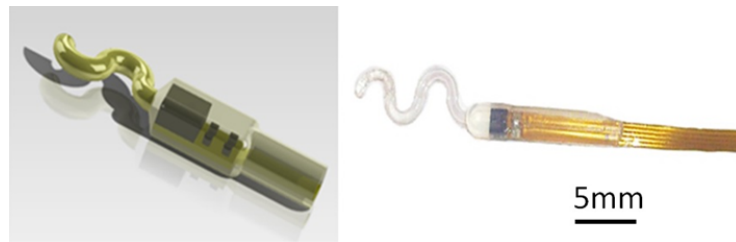
Figure 4.5: The heart muscle accelerometer device (version 1-1) with silicone encapsulation
