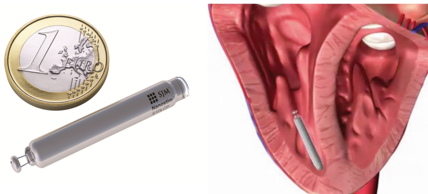
Figure 1.10: The Nanostim™ Leadless Pacemaker [62] (Overall length - Outer diameter: 42.3 mm - 6 mm). A Nanostim pacemaker stays within the right ventricle (to the right). Photos are reprinted with permission of St. Jude Medical, © 2015. All rights reserved.
