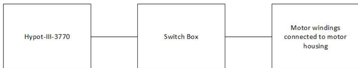
Figure 4. 1. 11: Insulation test scheme
