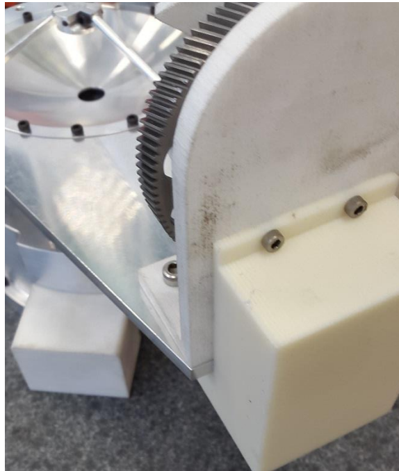
Figure 3. 12. 15: Motor house mounted to the bracket
