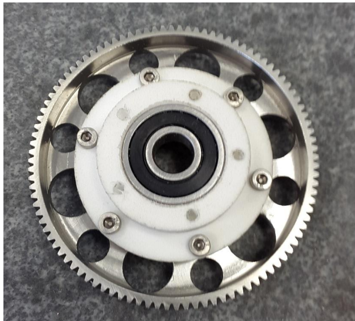
Figure 3. 12. 13: Gear mounted to bearing house elevation
