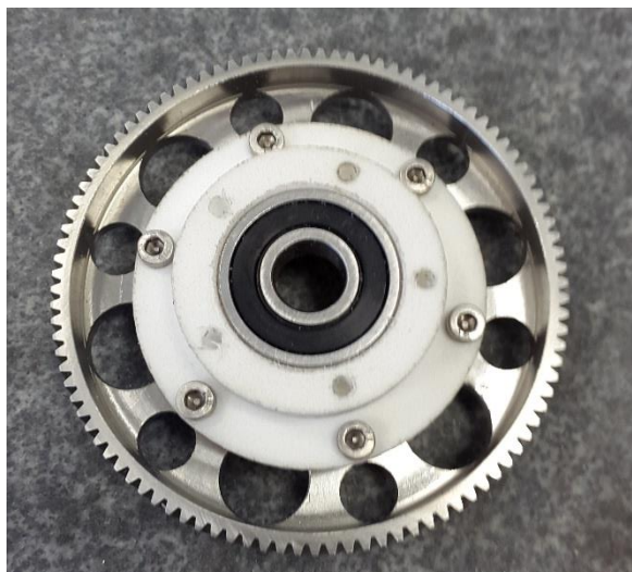
Figure 5.1.14: Gear on the elevation bearing house.
