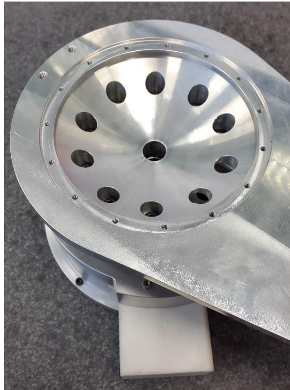
Figure 5.1. 9: Parabola holder and fishplate mounted on the azimuth stage.
