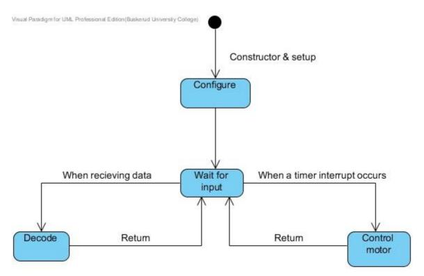
Figure 9: Motor Controller States
