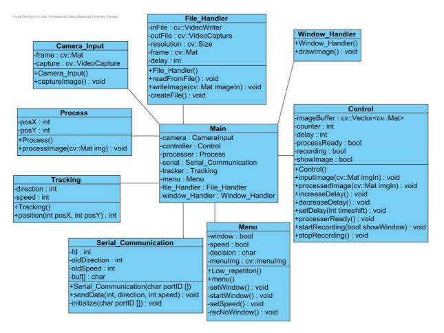
Figure 10: UML Class Diagram of Central Unit
