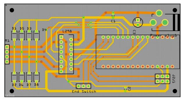
Figure 14: Proposed PCB layout designed in Fritzng
