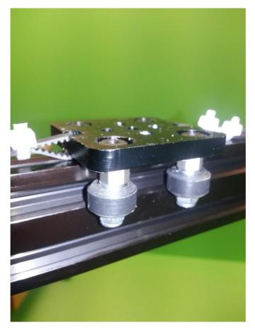
Figure 43: Camera Platform without camera housing
