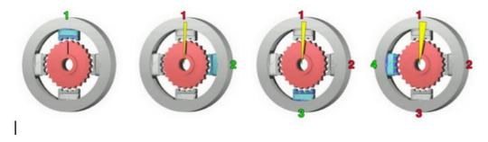
Figure 48: Full step one phase stepping principle, Source: <u>http://en.wikipedia.org/wiki/Stepper\_motor#cite\_note-2</u>
