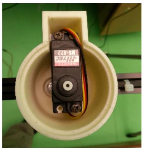
Figure 21: Servo House mounted on the Camera Rig
