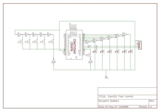
Figure 66: Circuit Schematic Foot Control
