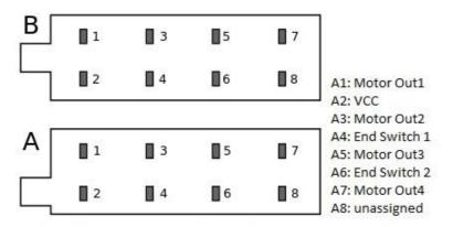
B2: GND B3: VCC B4: VCC B5: PAN B6: TILT B7: unassigned B8: unassigned
