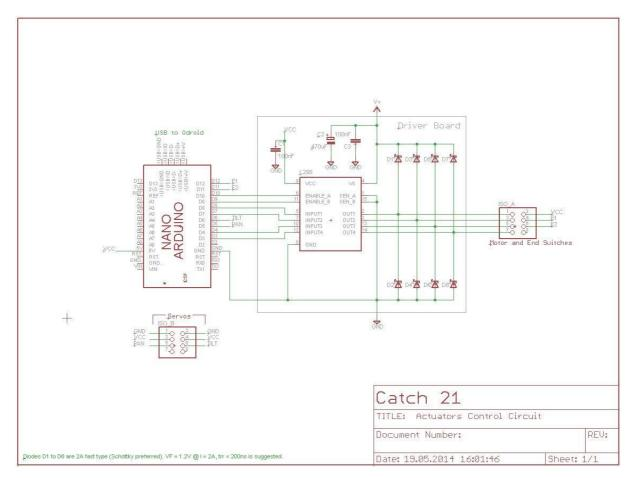
Figure 12: Control unit Schematic
