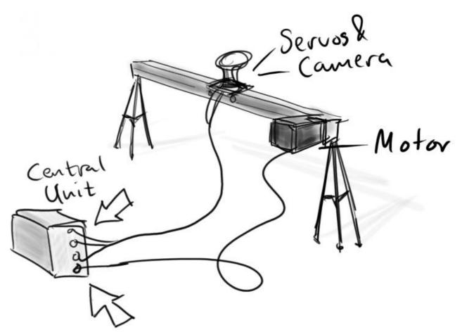
Figure 32: Concept Drawing Central Unit & Rig
