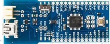
Figure 70: The Arduino Fio
