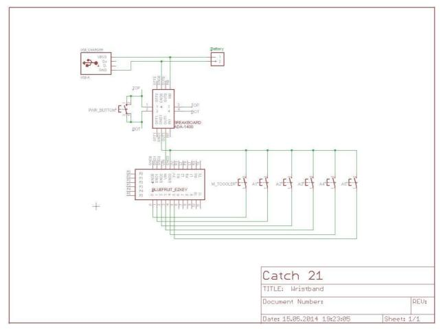
Figure 71: The Wristband Circuit Schematic
