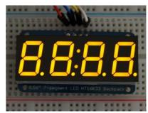
Figure 64: 4-Digit 7-Segment Display with a Driver backpack
