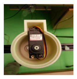
Figure 53: 3D-printed casing with the pan-servo
