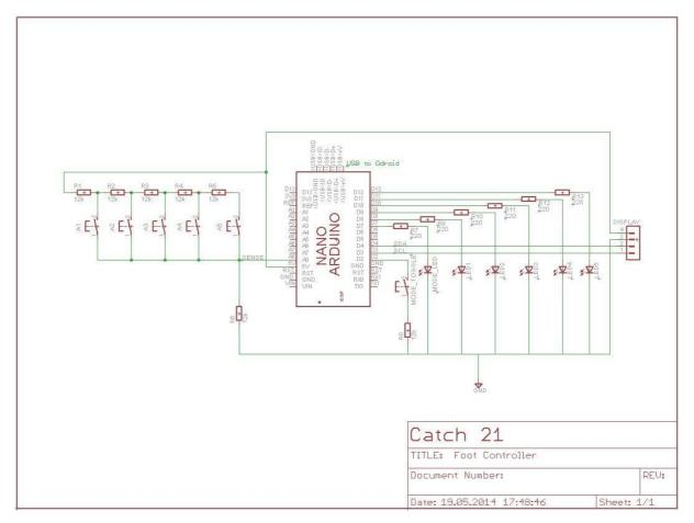
Figure 15: Foot controller schematic
