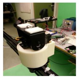
Figure 54: The mount for the camera and the tilt-servo
