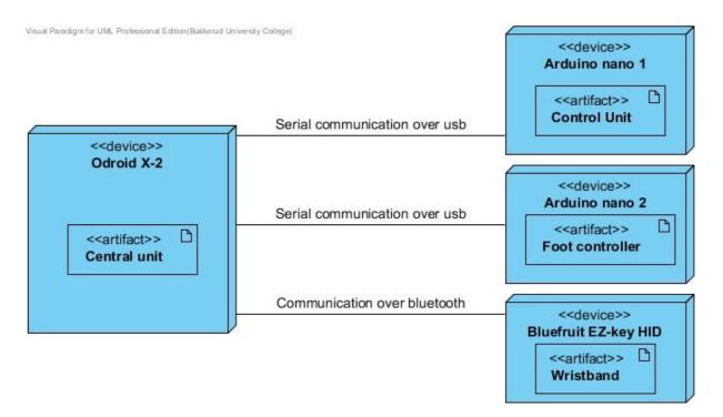
Figure 7: Processing Devices
