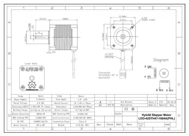
Figure 46: Stepper Motor Specification Datasheet. Source: Open Builds [1]
