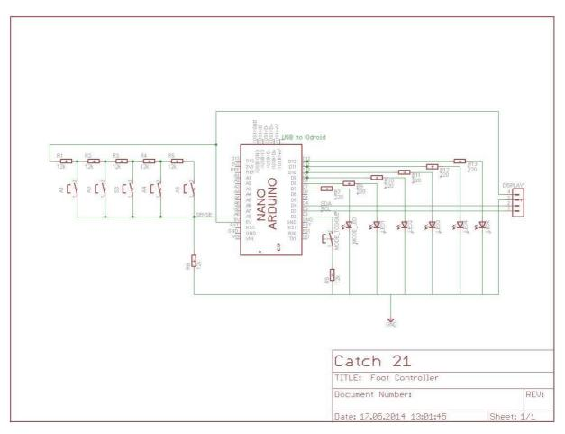
Figure 75: Foot Controller Schematic
