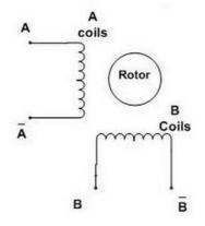
Figure 47: Bipolar Stepper Motor Wiring Diagram
