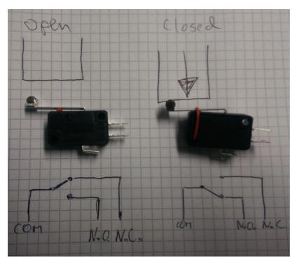
Figure 56: End stop switches
