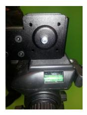
Figure 55: The tripod is connected to the rig endmount
