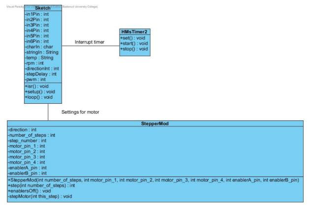
Figure 11: Control Unit Class Diagram
