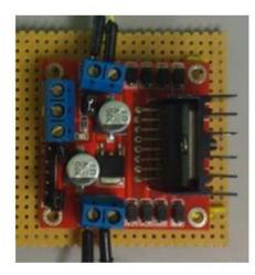
Figure 51: L298 Dual H-Bridge Motor Driver
