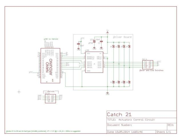
Figure 74: Actuators Schematic
