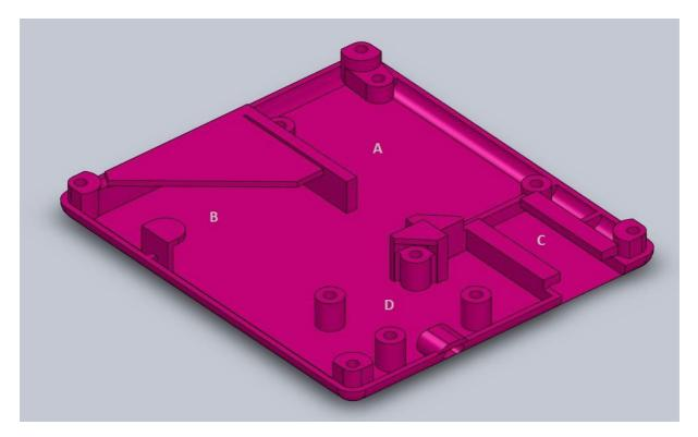
Figure 19: Bottom plate featuring deadicated slots & sockets for: A:Bluefruit Ez-Key, B:Battery, C:Charger, & D:On/Off Switch
