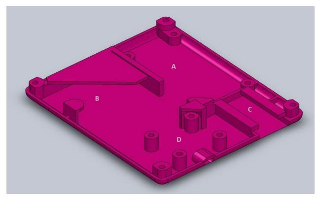
*Figure 72: The 3D design of the bottom plate with sockets for: A: Bluefruit Ez-Key B: Battery Slot C: Charge pin sleeve D: On/off button*
