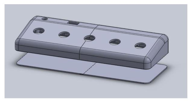
Figure 17: Assembly view of the Foot Controller casing
