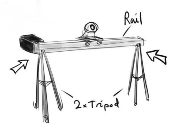
Figure 31: Concept Drawing Rig (Motor, camera and servos come attached to the rail.)
