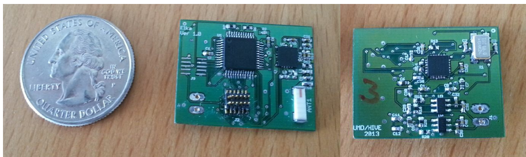
Figure 23. The fully assembled Elka Board compared with a quarter of dollar.
