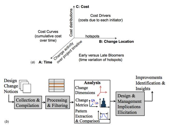
Fig. 1.4 (a) Dimensions of engineering change and (b) engineering design change analysis process
