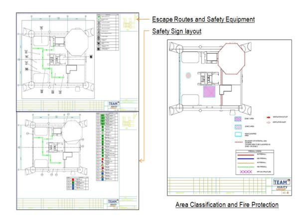
Fig 6.5 Sample of Safety sign layout, escape route and safety equipment & area classification 2D Drawing
