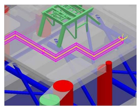
Fig 6.3 Sample of 3D Escape route model from SmartPlant
