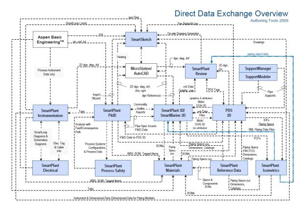
Fig. 4.5 SmartPlant Direct Data Exchange overview [35]
