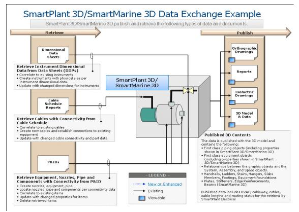
Fig. 3.8 SmartPlant 3D/SmartMarine 3D Data exchange example [35]
