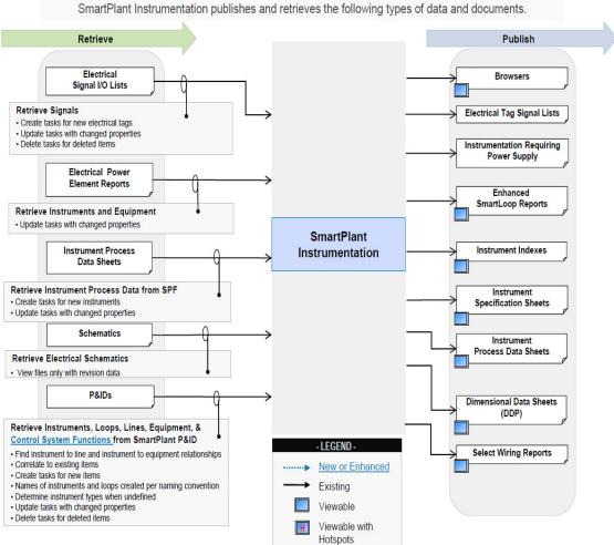
SmartPlant Instrumentation Data Exchange Example
