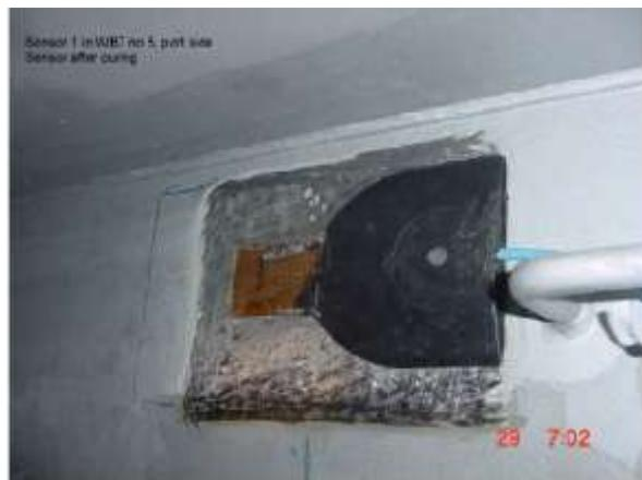
*Figure 3. 2: A photo of a sensor package glued on a stiffener before coating (Light Structures, Installation manual)*
