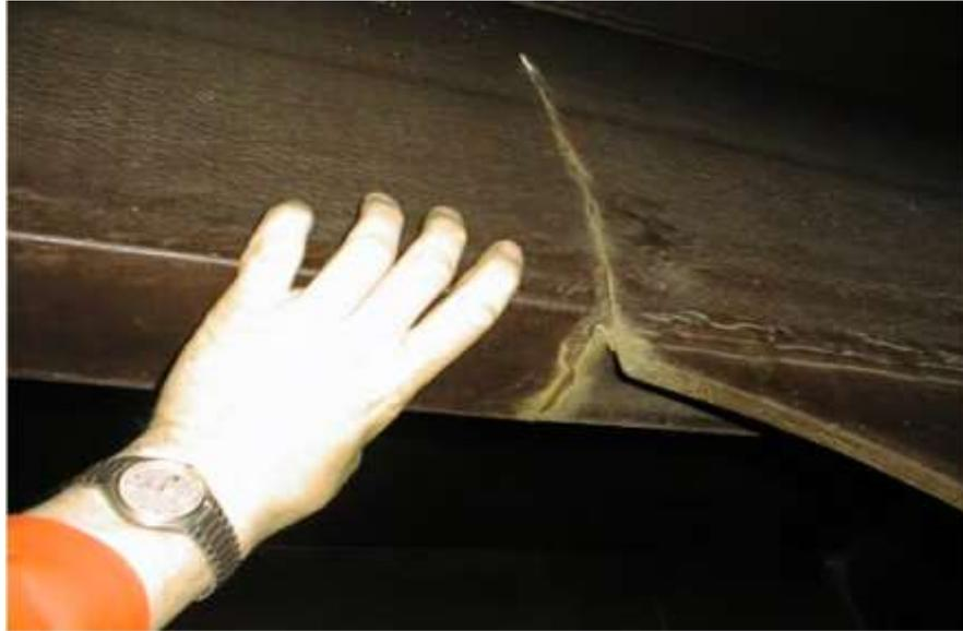
**Figure 1 2:** Picture of a longitudinal stiffener in deck in way of the transverse bulkhead in a large blunt ore carrier. The crack originated from the bracket toe termination after one year of operation (Storhaug G. , 2007).
