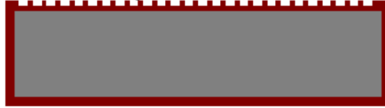
Figure 4.4 RIE etch of the cavities
