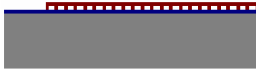
Figure 4.9 Etching access to the bottom electrode
