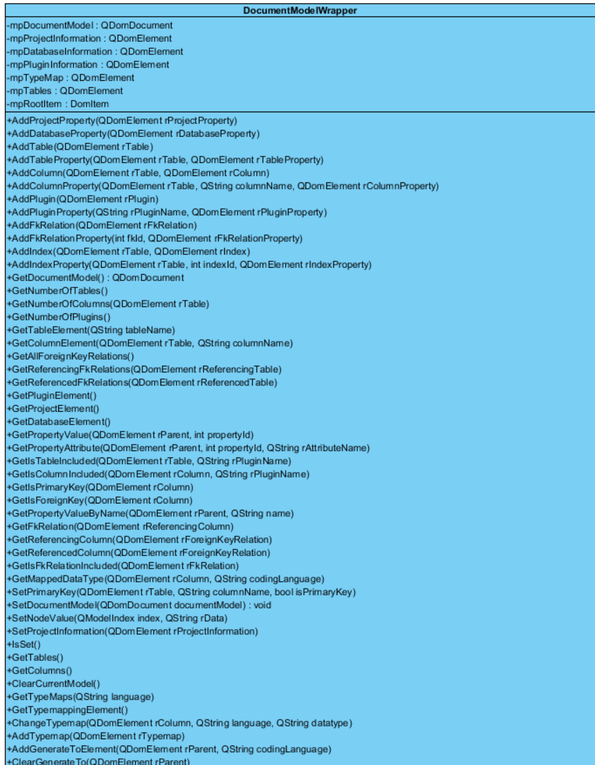
Figur 10: Klassediagram for DocumentModelWrapper (del 1/2)
