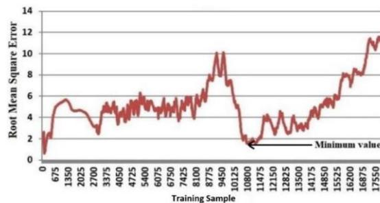
Figure 10. RMSE values for different training sample number values for short-term forecasting.
