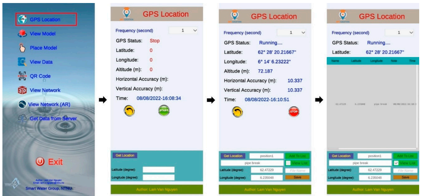
Figure 10. Pinpointing locations using GPS signals.
