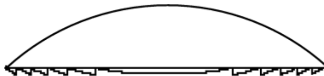
Figure 2 Combination of refractive and diffractive hybrid lens [4]
