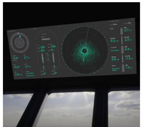
Figure 14. Example of how compass, thrusters and RADAR can be presented in AR (Courtesy of AHO and SEDNA).
