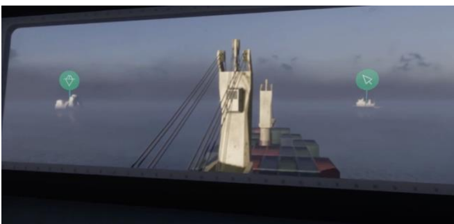
Figure 11. Example of how markings of dangers and traffic can be presented in AR (Courtesy of AHO and SEDNA).
