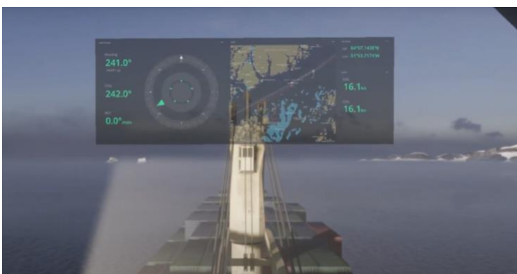
Figure 13. Example of how compass, speed and ECDIS information can be presented in AR (Courtesy of AHO and SEDNA).
