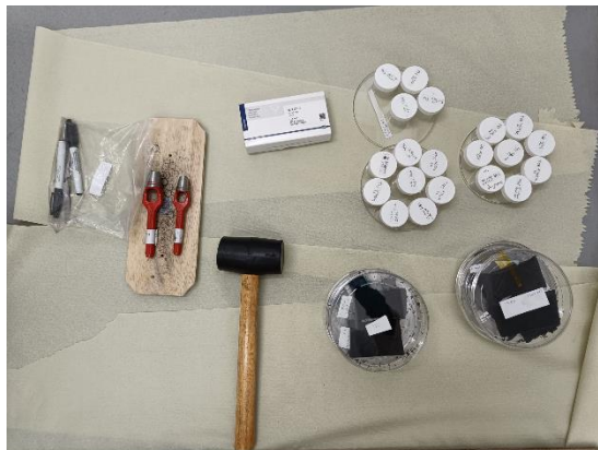
Coin Cell Electrode Sizing & Preparation
