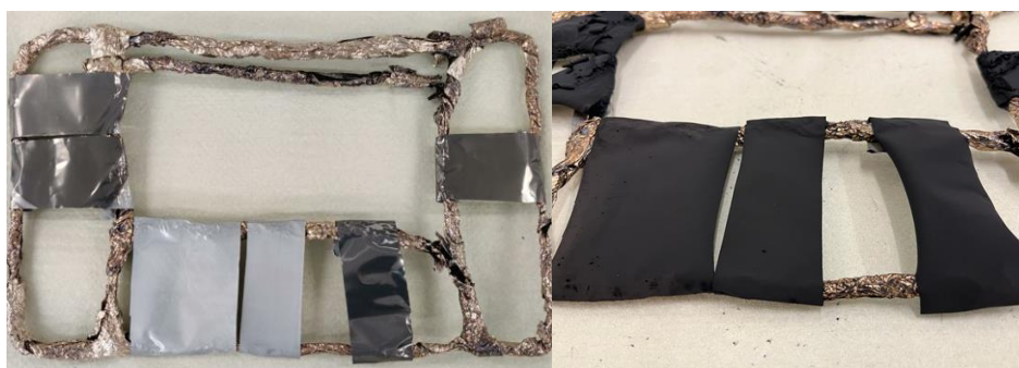
Figure 3-2: Typical samples before and after the growth of CNTs
