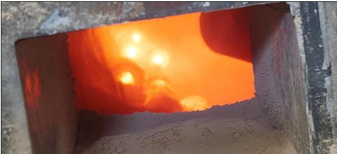
Figure 6.7: Snapshot of broken heating elements rolling inside the calciner during the tests with cement raw meal.
