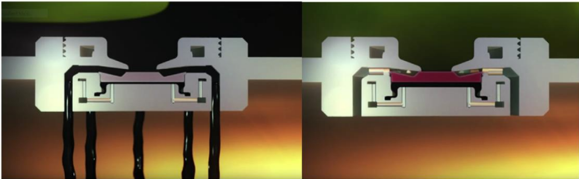
Figure 2.18: AICV open position (left) and closed position (right) [54].
