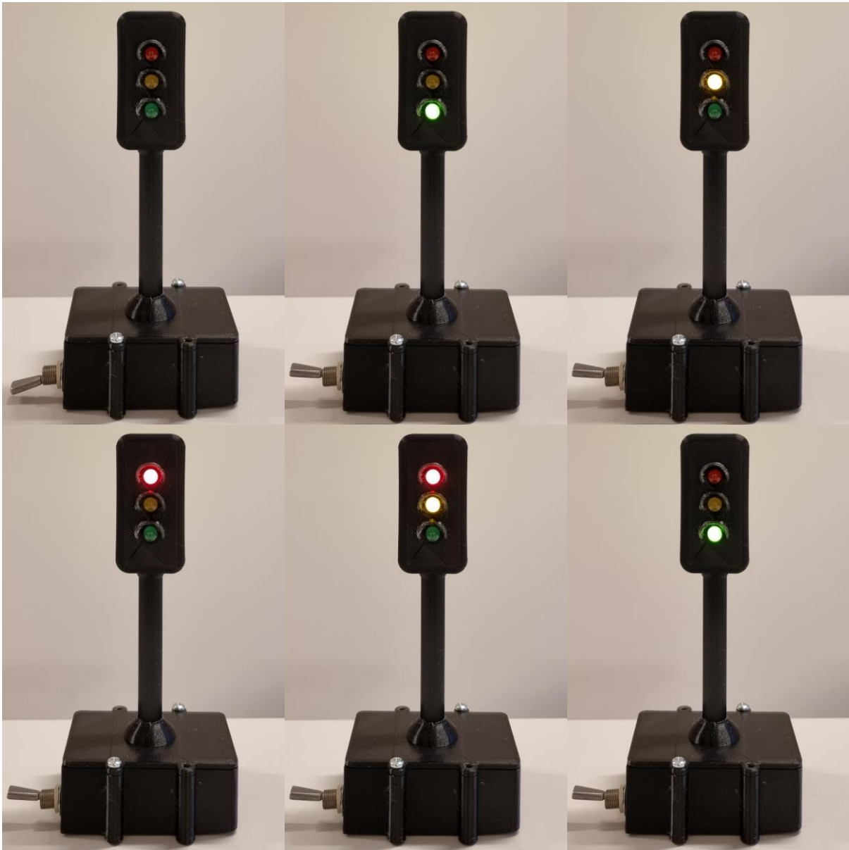
Figure 2.7: Finished traffic light, complete color sequence.
