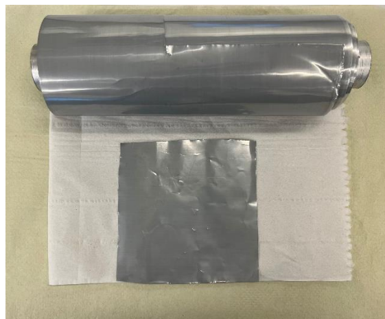
Figure 3-2: pre-etched 70 \mu\text{m} Al Foil.
